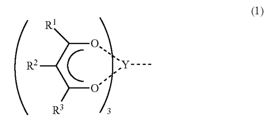
where R<sup>1</sup>, R<sup>2</sup>, and R<sup>3</sup> represent hydrogen or a substituent group with 1 to 12 carbon atom/s, 0 represents an oxygen atom, and Y represents an yttrium atom.
