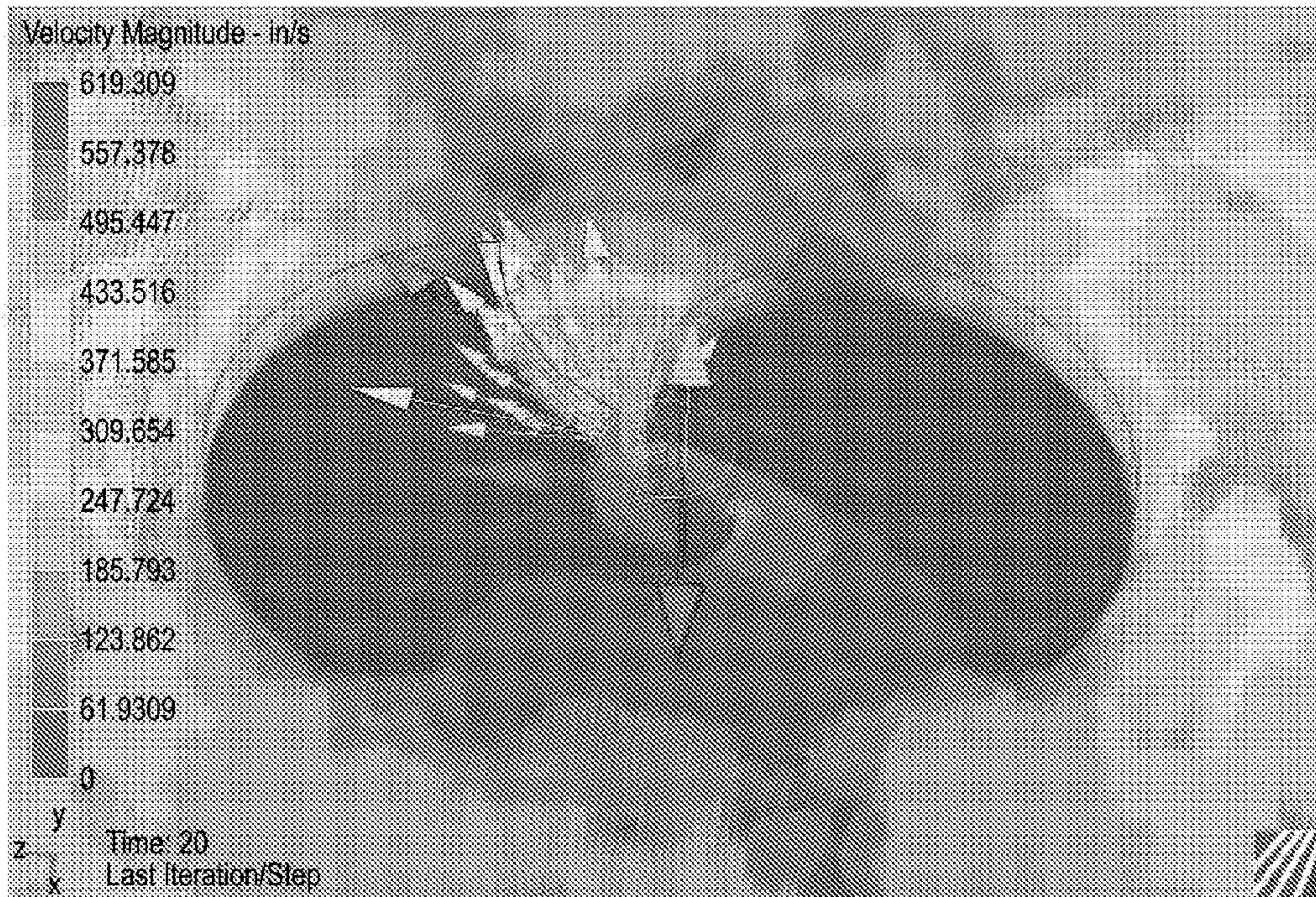
Figure 19: Energy distribution in concentrating funnel.
