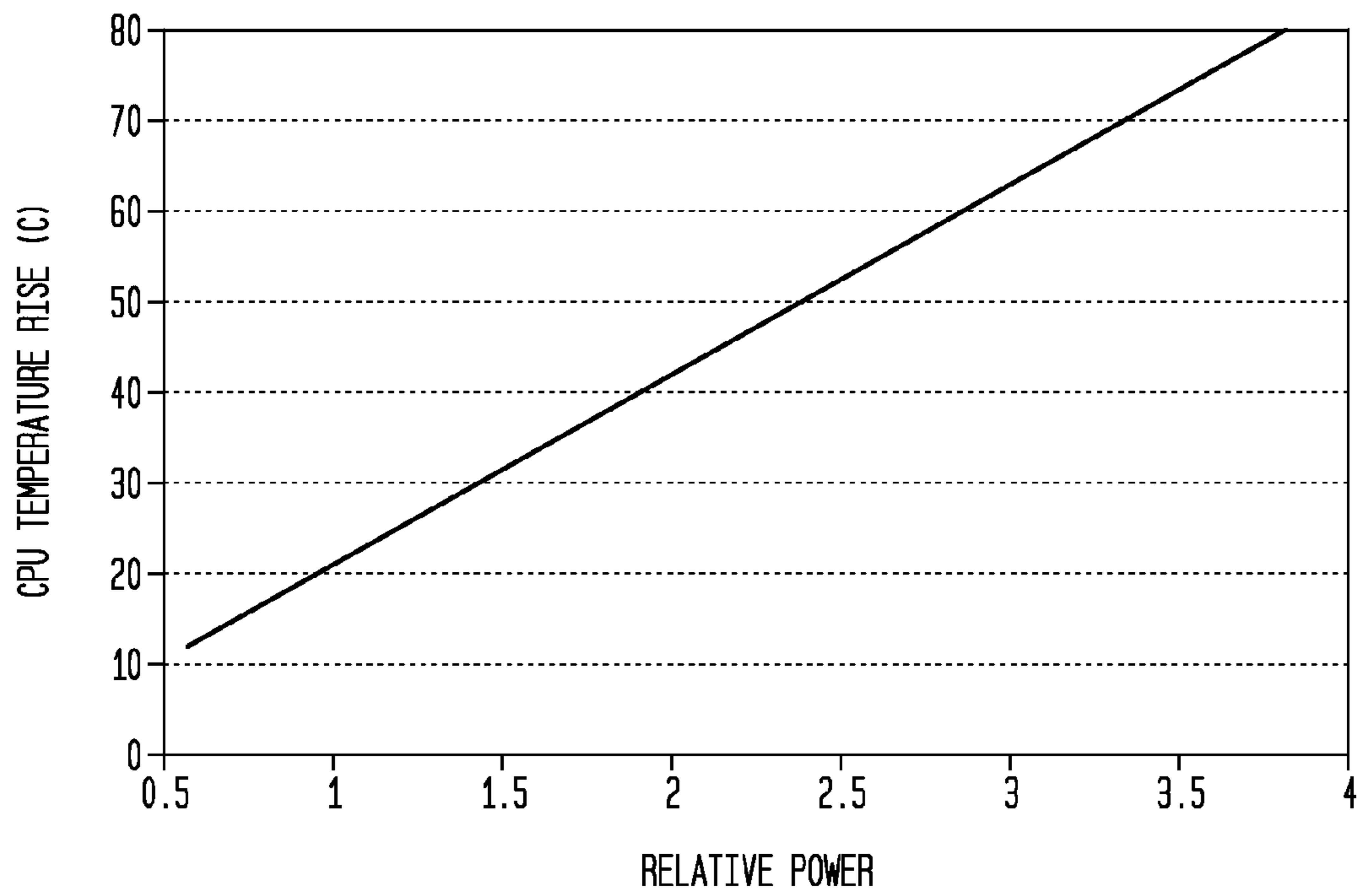
CPU TEMPERATURE VS. POWER
