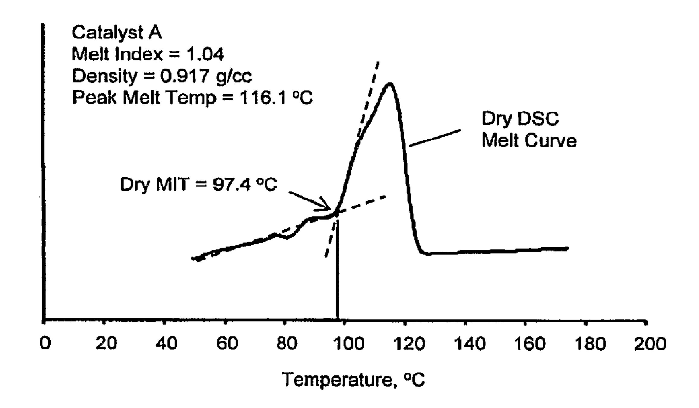
Figure 4 – Displaced MIT (MIT<sub>R</sub>)
