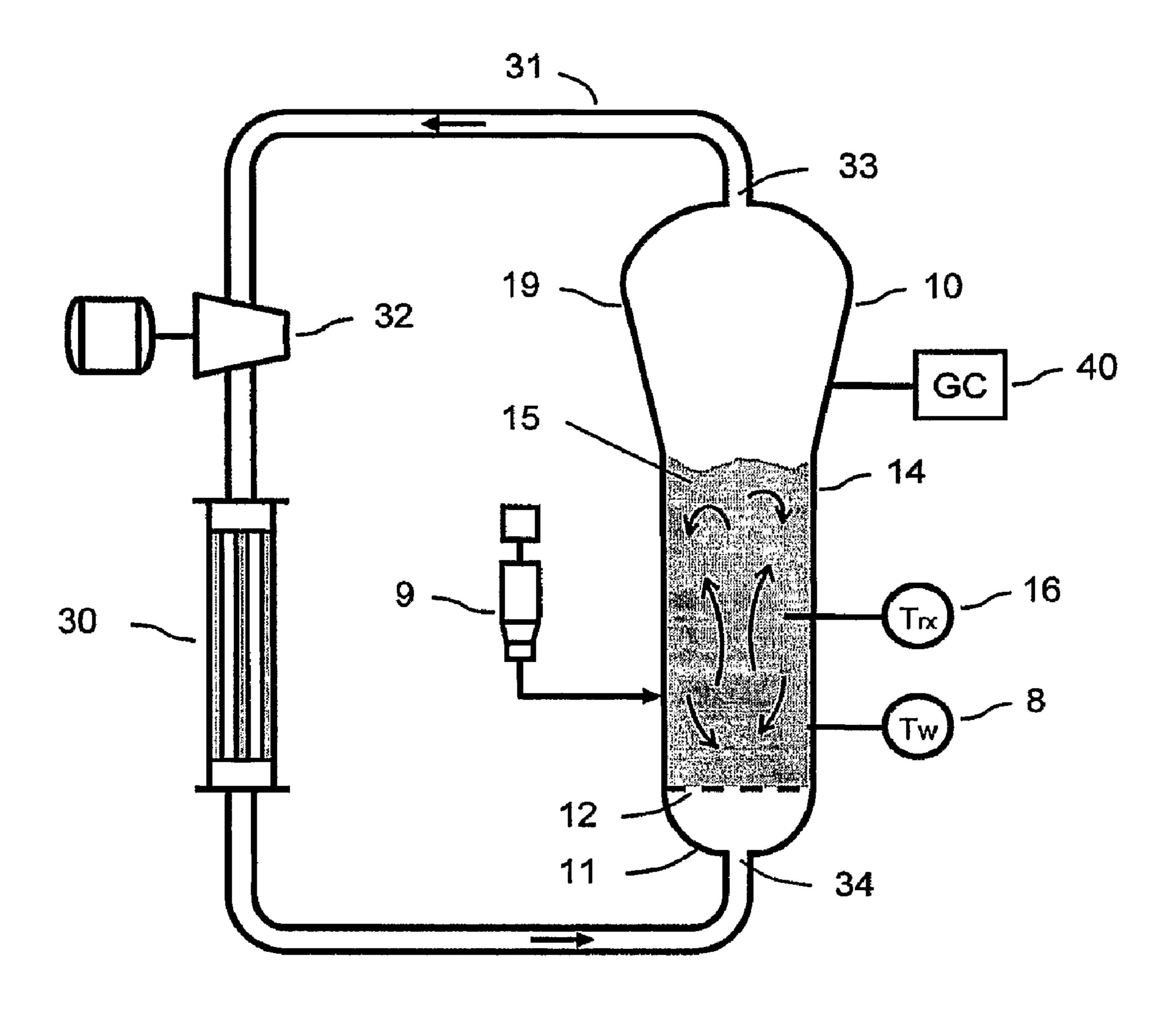
Figure 2 – Process For Monitoring And Control of Reactor Stickiness
