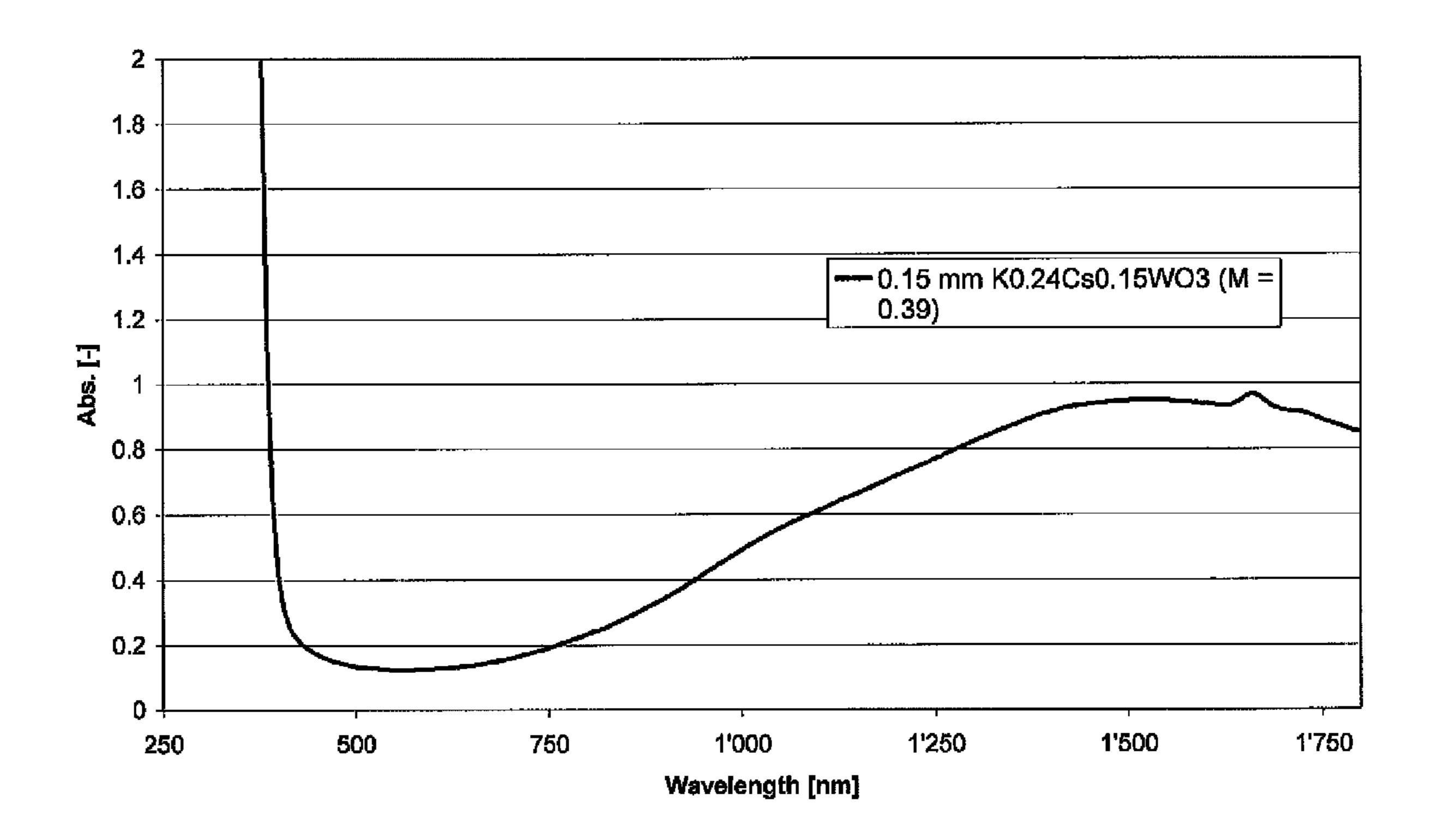
Fig. 2: UV-VIS-NIR-Spectrum of K<sub>0.24</sub>Cs<sub>0.15</sub>WO<sub>3</sub> in plasticized PVB 1 mm plaque
