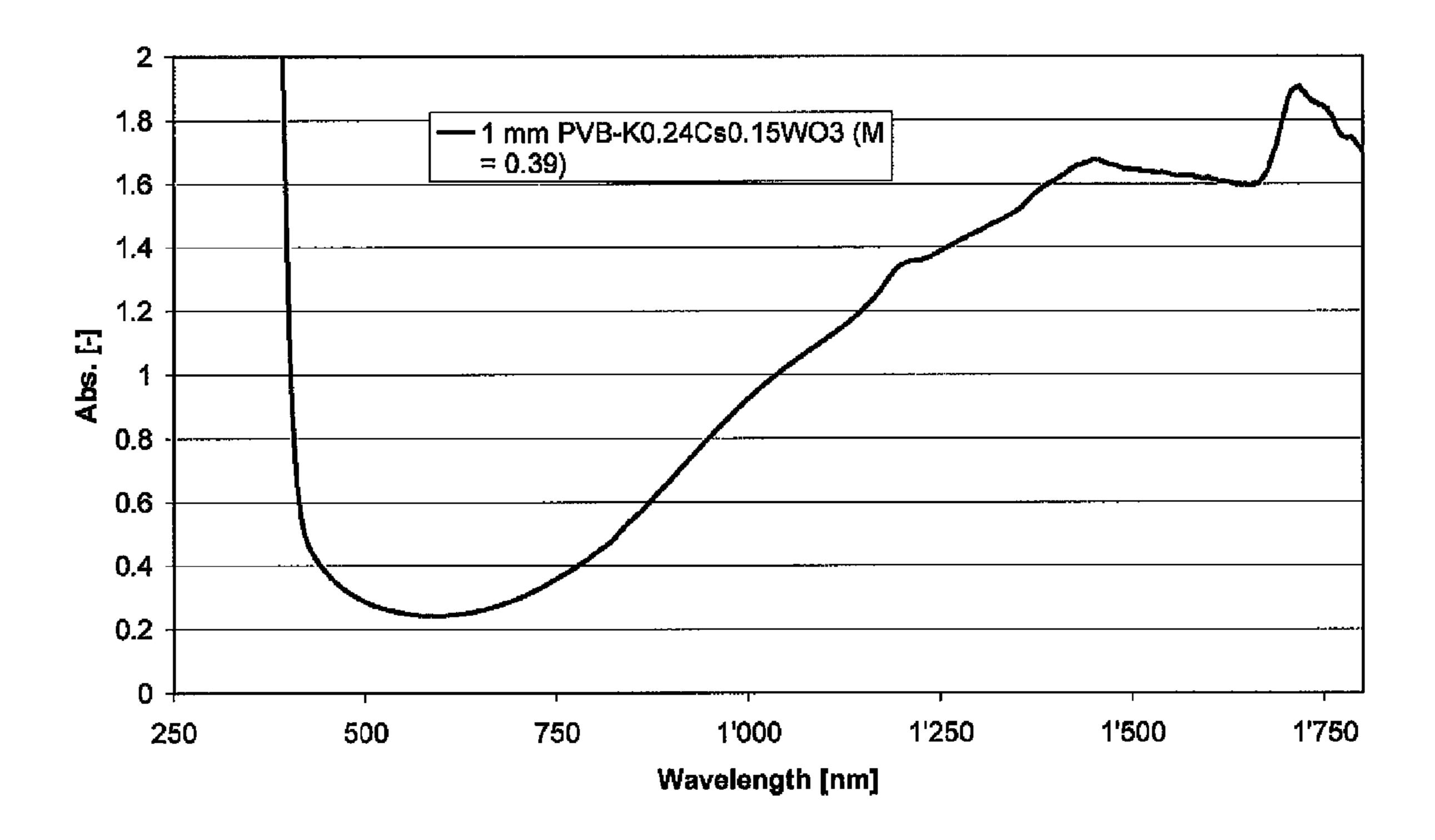
Fig. 3: UV-VIS-NIR-Spectrum of  $K_{0,24}Cs_{0,15}WO_3$  in 0.45 mm PVC film
