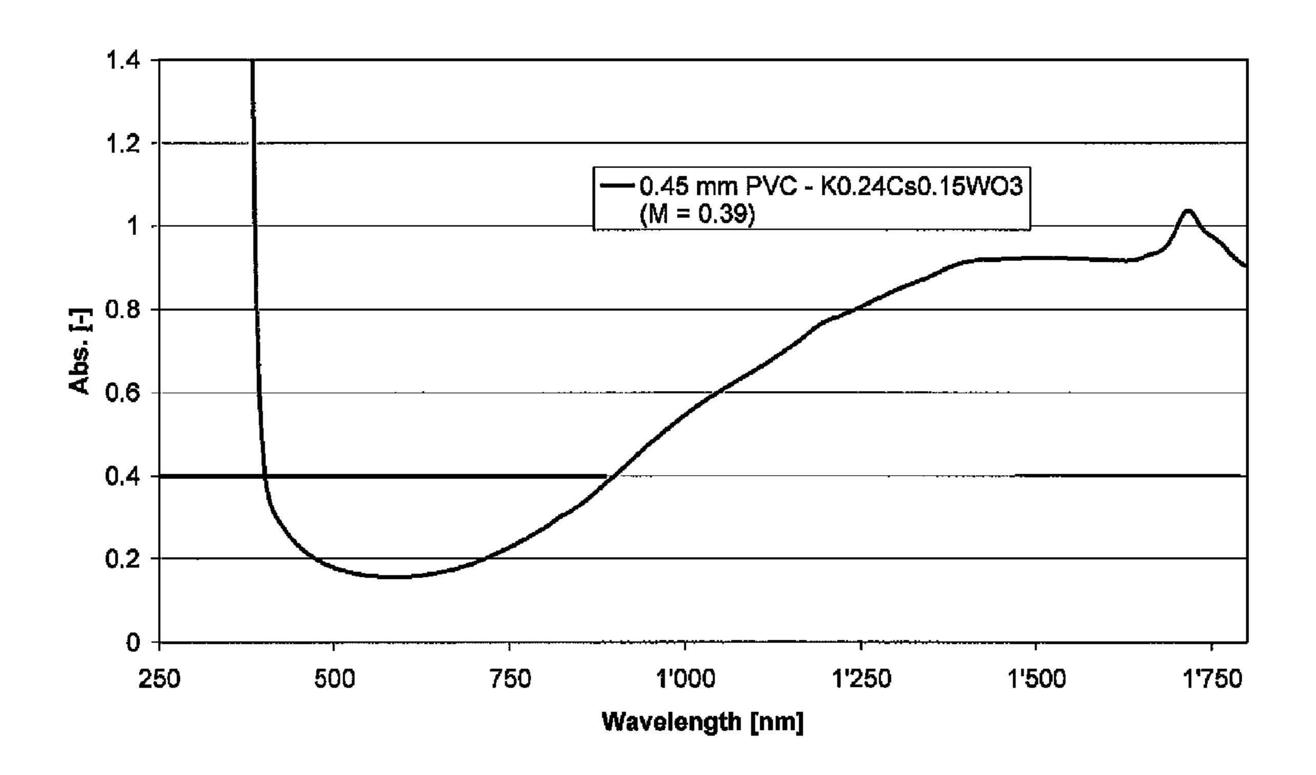
Fig. 4: UV-VIS-NIR-Spectrum of K<sub>0.24</sub>Cs<sub>0.15</sub>WO<sub>3</sub> 0.1 mm PC film
