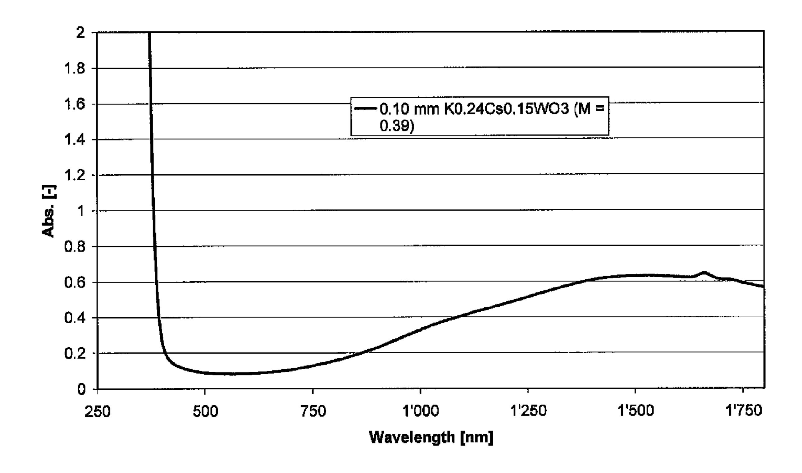
Fig. 5: UV-VIS-NIR-Spectrum of K<sub>0,24</sub>Cs<sub>0,16</sub>WO<sub>3</sub> 150 micron LDPE film
