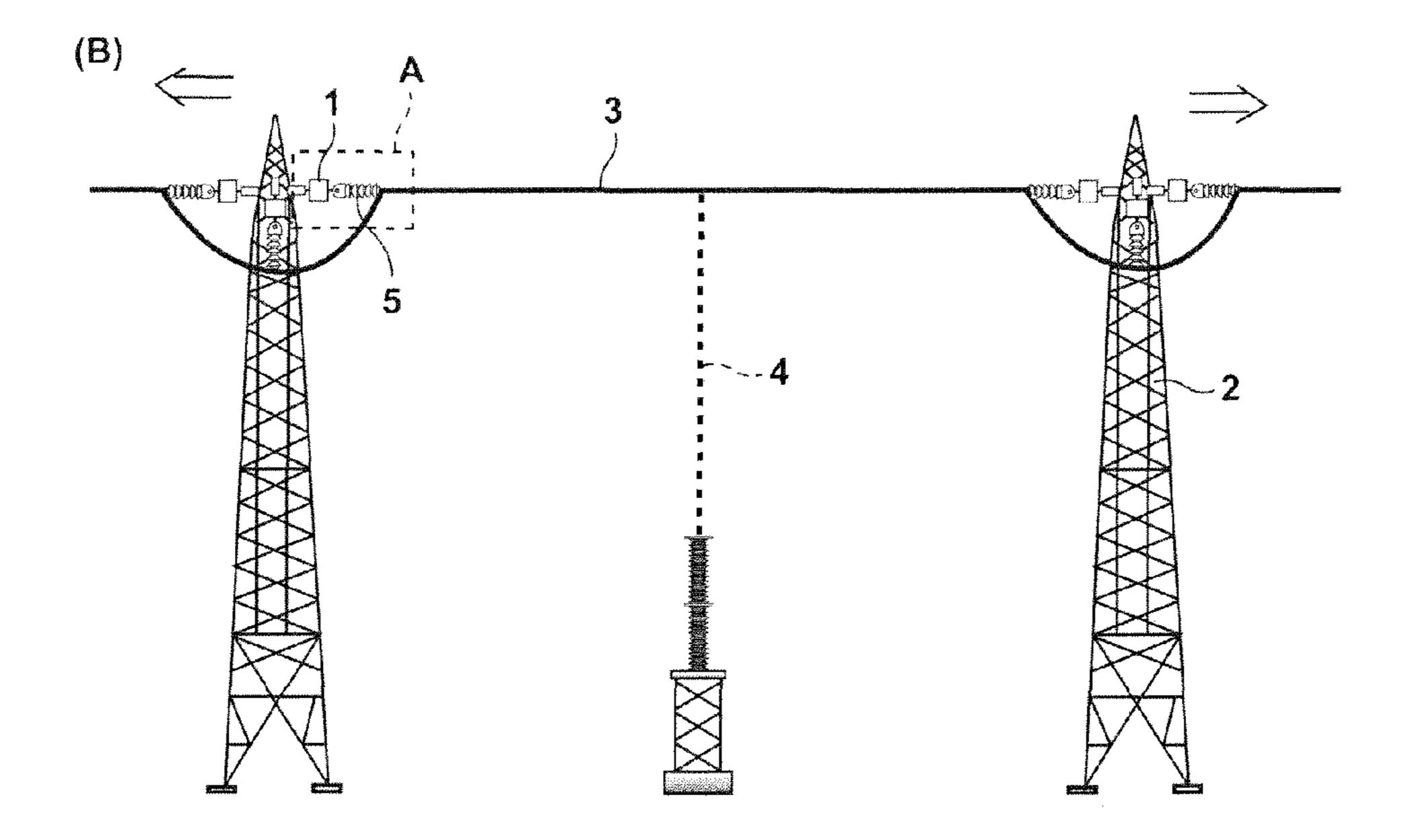
The power line tension balancer related to one embodiment of the present invention is installed.
