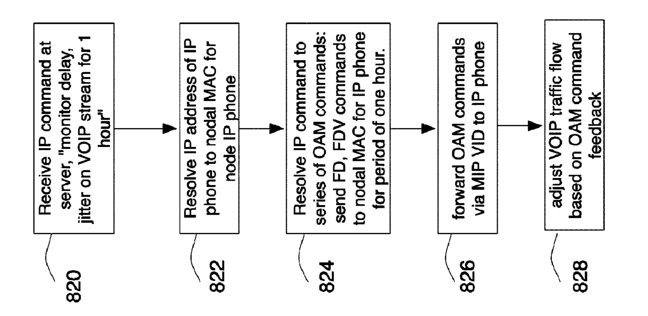
access pox 802 delay, jitter Figure 17 806 808 monitor bridge server
