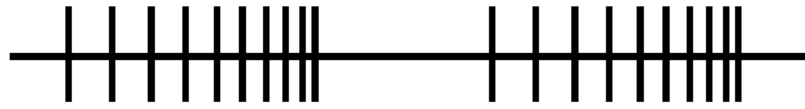
Figure 11a Chirped Gratings. Fabry-Perot like modulator composed of two chirped gratings for multi-peak periodic spectra
