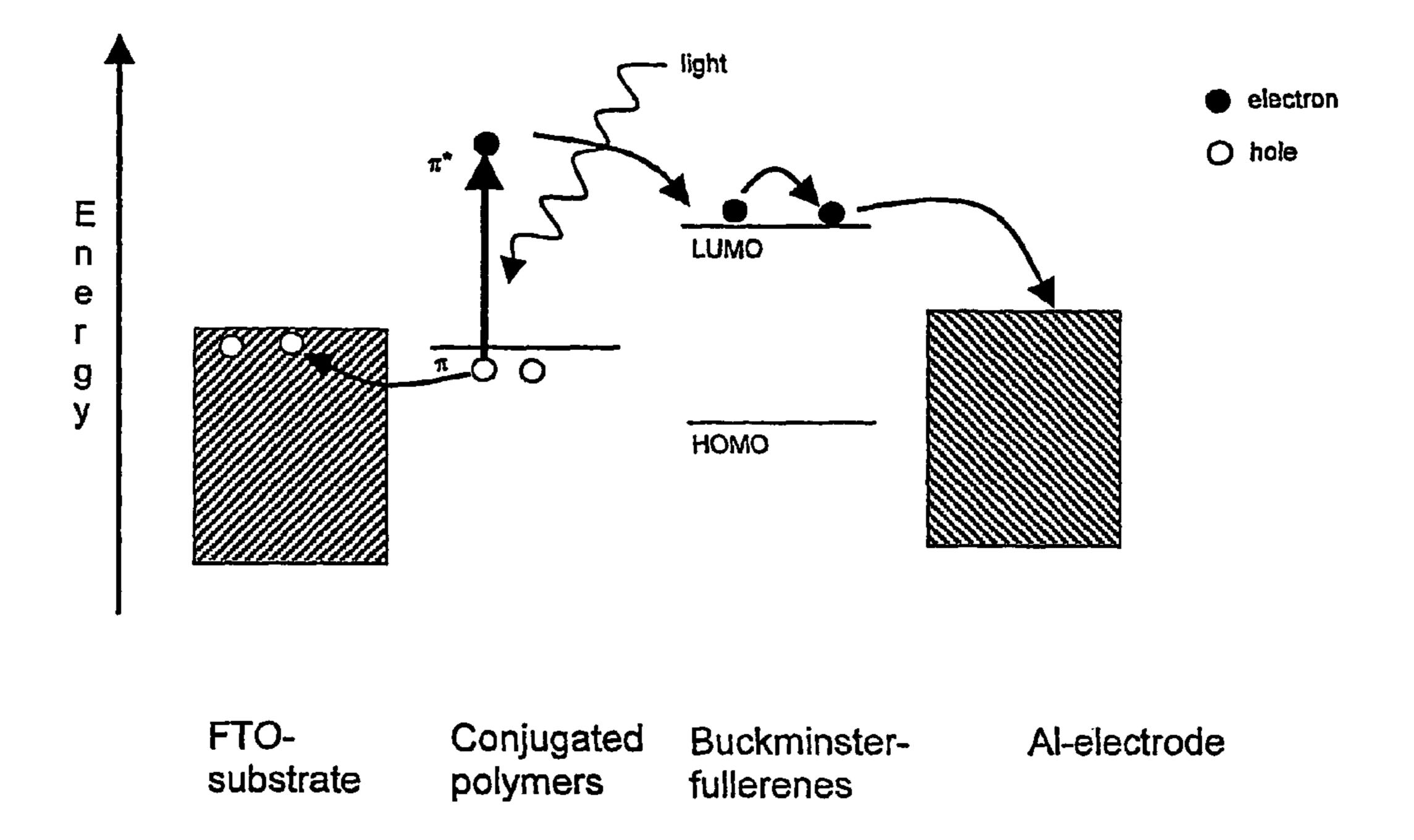
Fig. 1: Schematic band diagram and different excitation processes of and in solar cells based on Buckminsterfullerenes.
