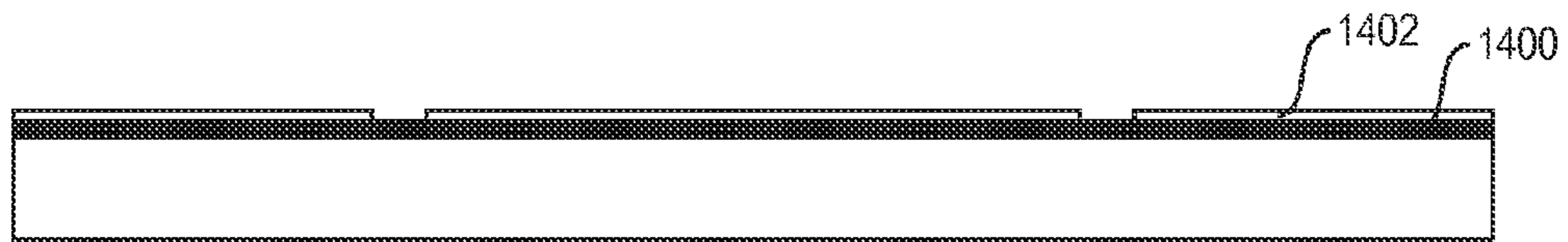
1ST PARYLENE DEPOSITION AND PATTERNING (MASK #1)
