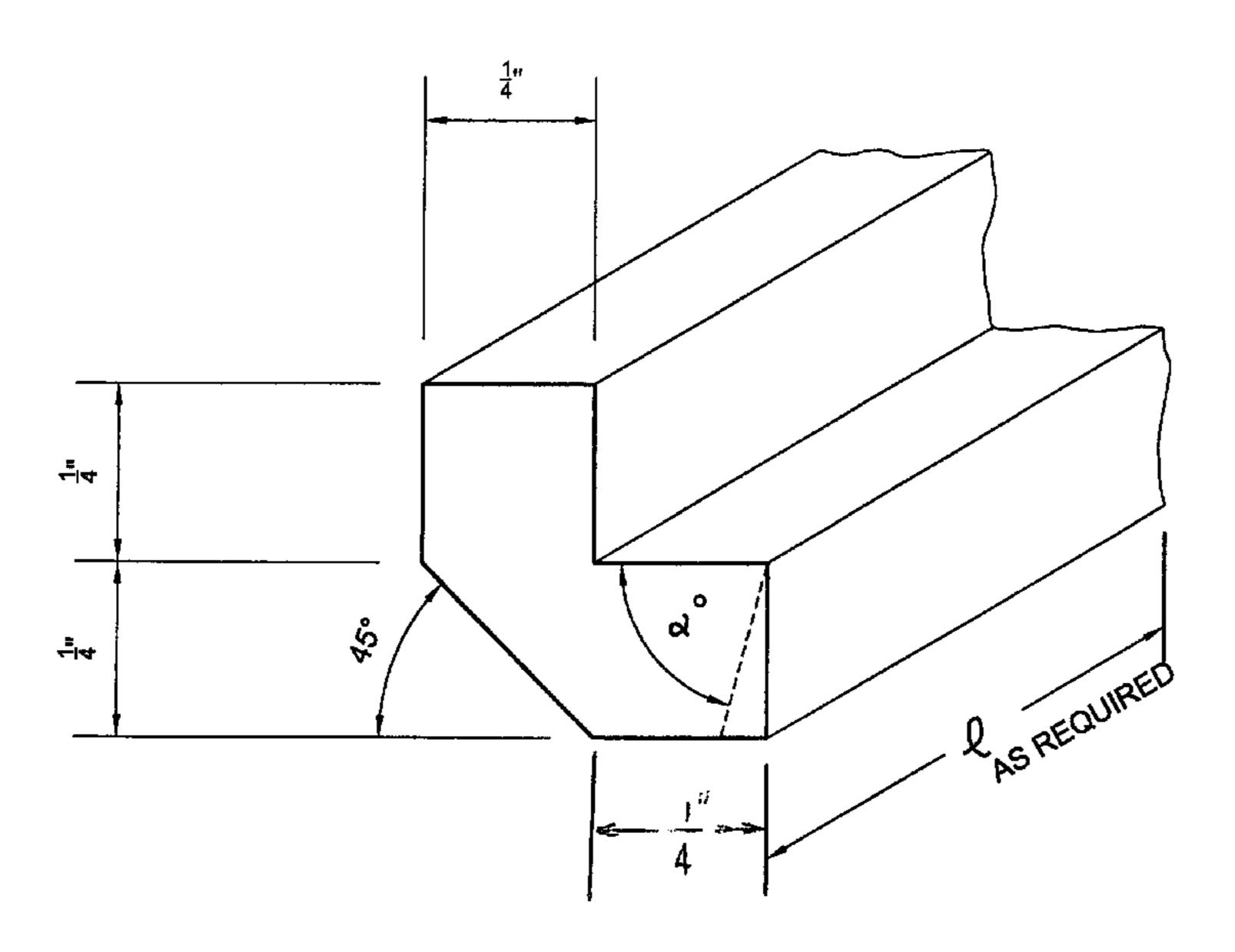
$a^{\circ} = 75^{\circ} \pm 15^{\circ}$  AS REQUIRED
