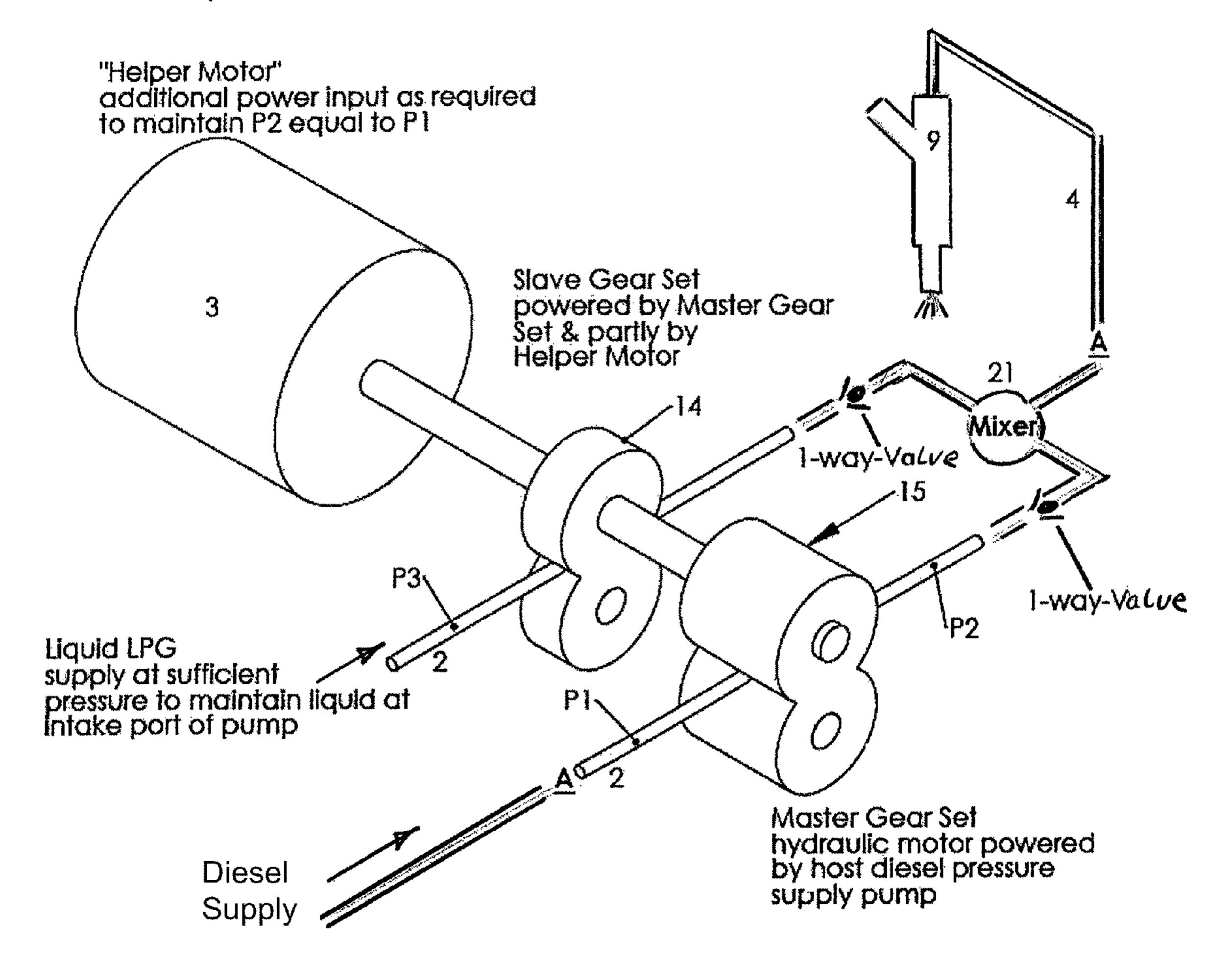
The pressure loss P1 to P2 is due to energy lost in driving slave pump, additional electrical energy is required to raise P2 to equal P1
