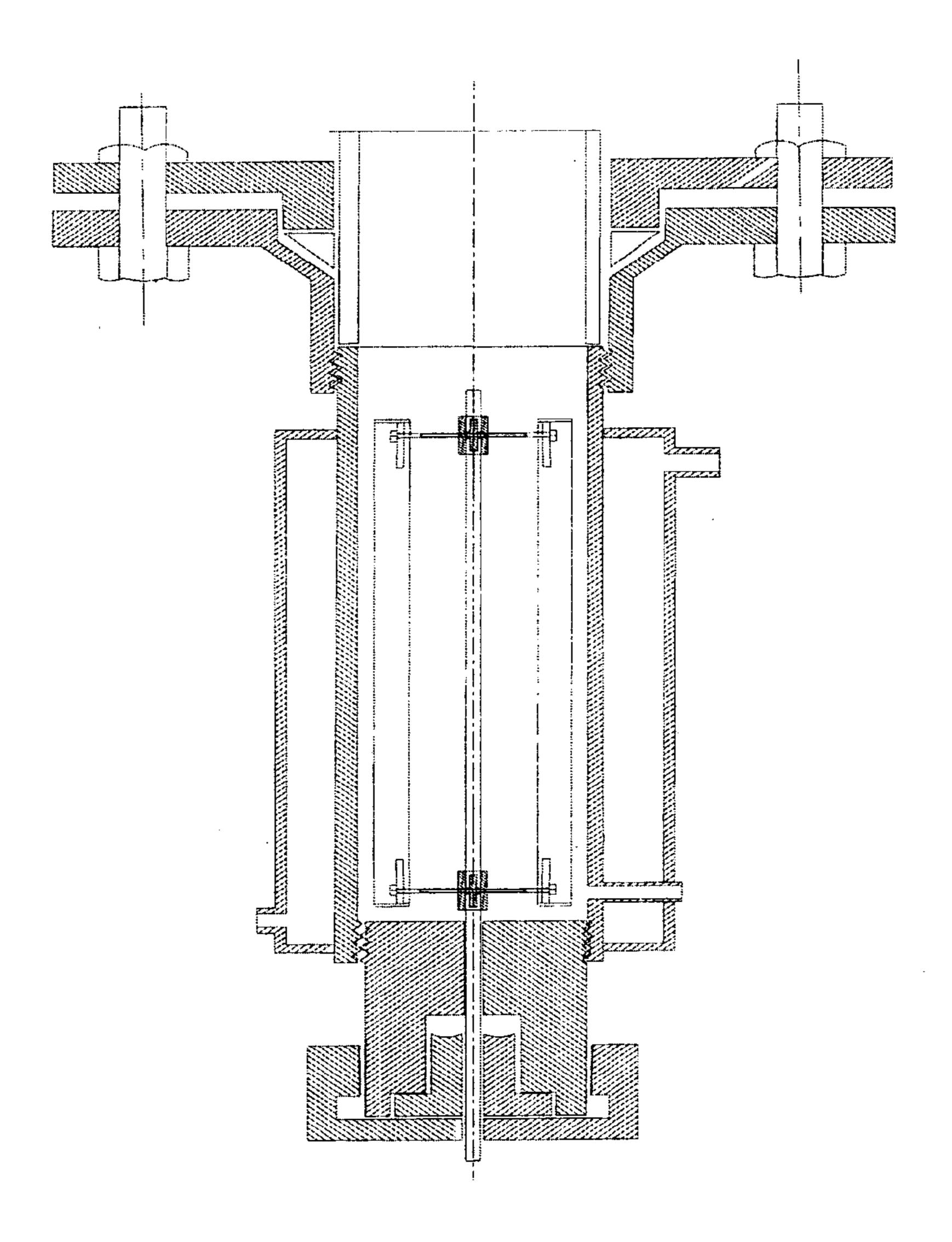
Figure: 2 shows the section of freezing concentration column where the step 1 is happened. This portion consist jacket for circulation of refrigerant, and scraper which help for scraping of ice.
