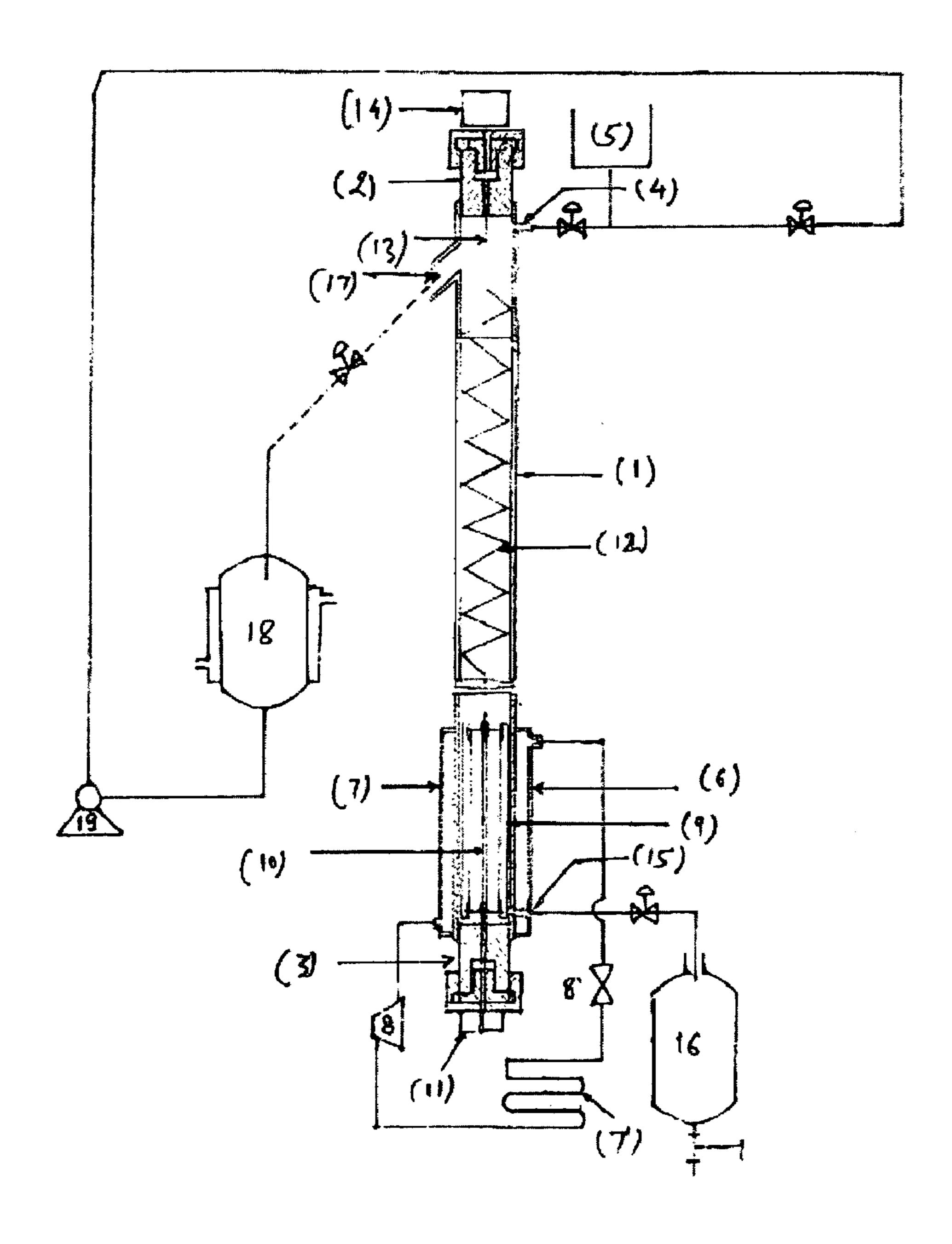
Fig.1: Schematic diagram of fractional freeze column with external attachments
