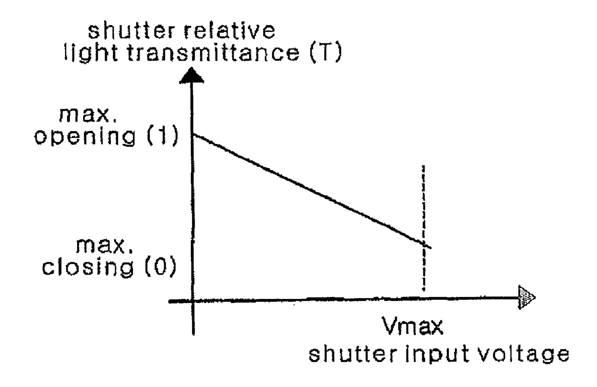
shutter input voltage corresponding shutter O/C sequence state value
