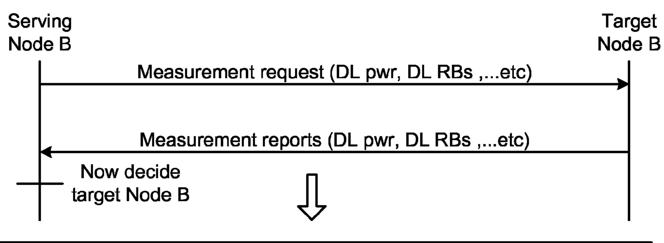
To ensure HO success serving Node B needs to know all target Node B measurements leading to signalling wastage if HO not possible
