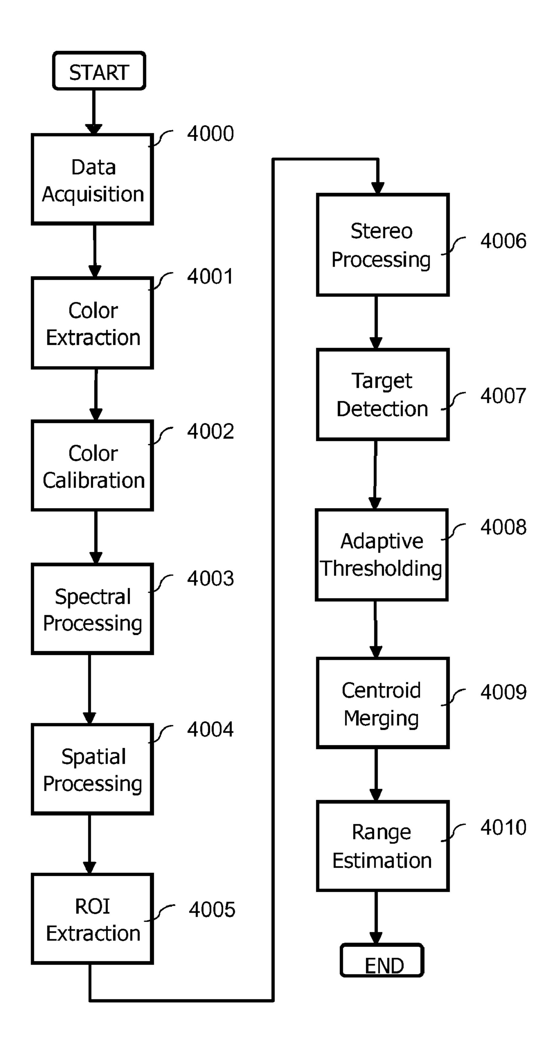
Figure 4. Drowning detection processing
