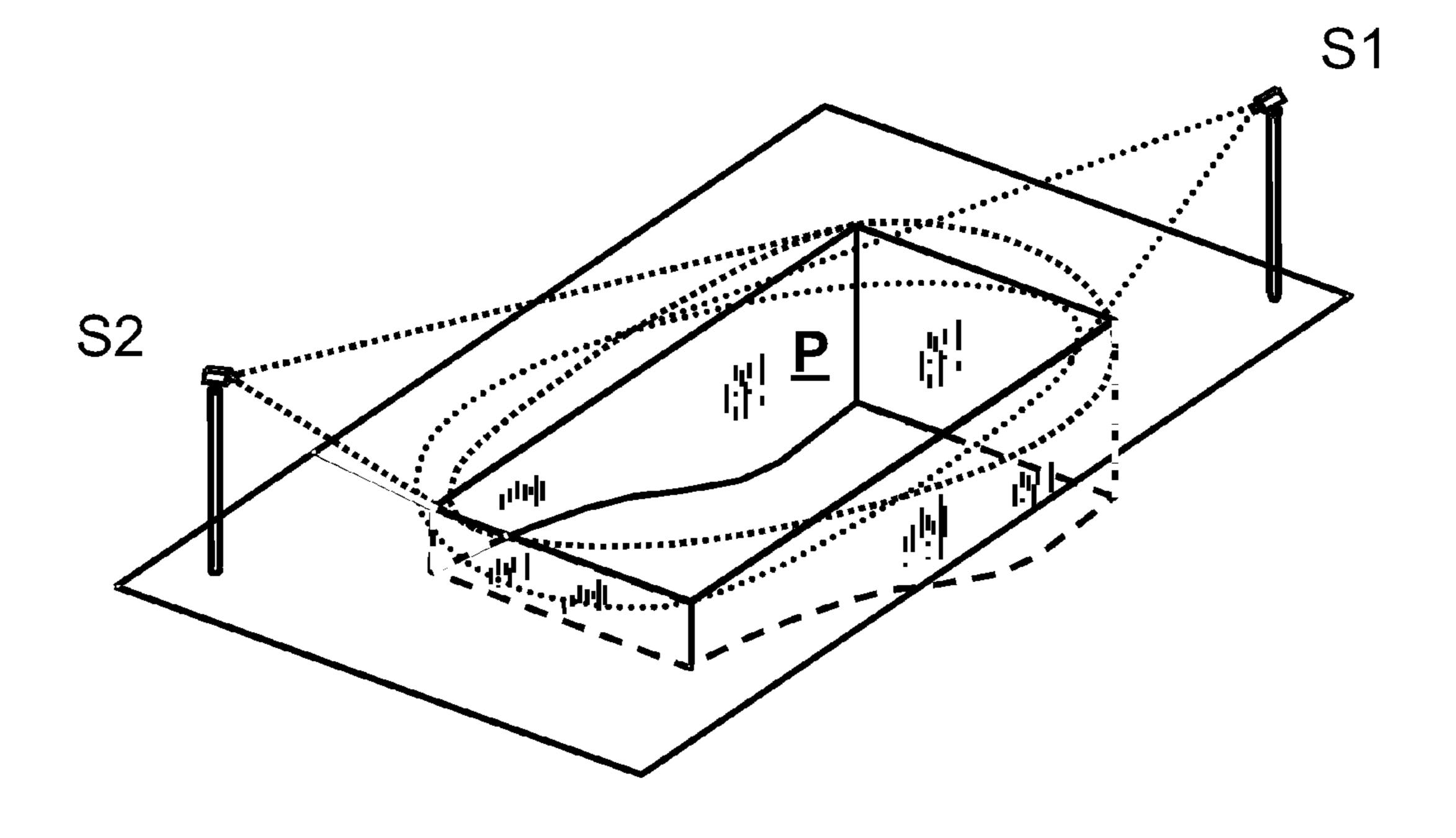
Figure 1. Pool Monitoring Sensor Configuration
