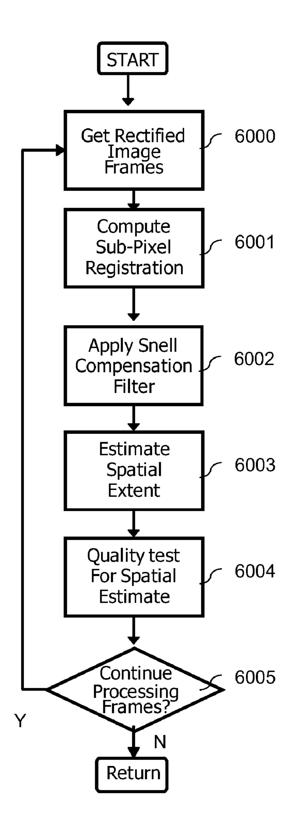
Figure 6. Processing steps for performing stereo processing
