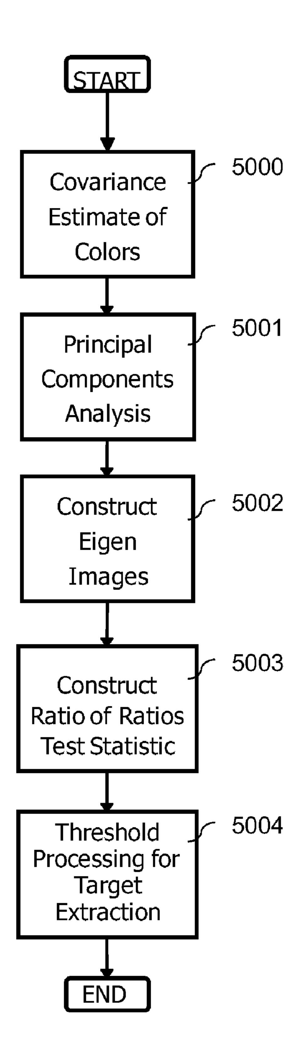
Figure 5. Processing steps for performing spectral processing
