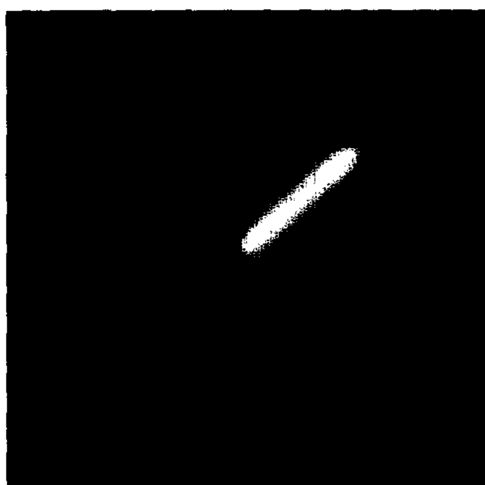
Figure 24. Opaque (97% attenuation) coded aperture image at a maximum pixel count of 3270, 10 minutes
