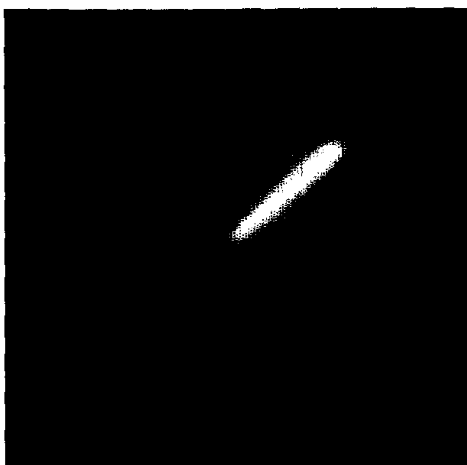
Figure 23. Opaque (97% attenuation) coded aperture image at a maximum pixel count of 286, 45 seconds, showing some noise
