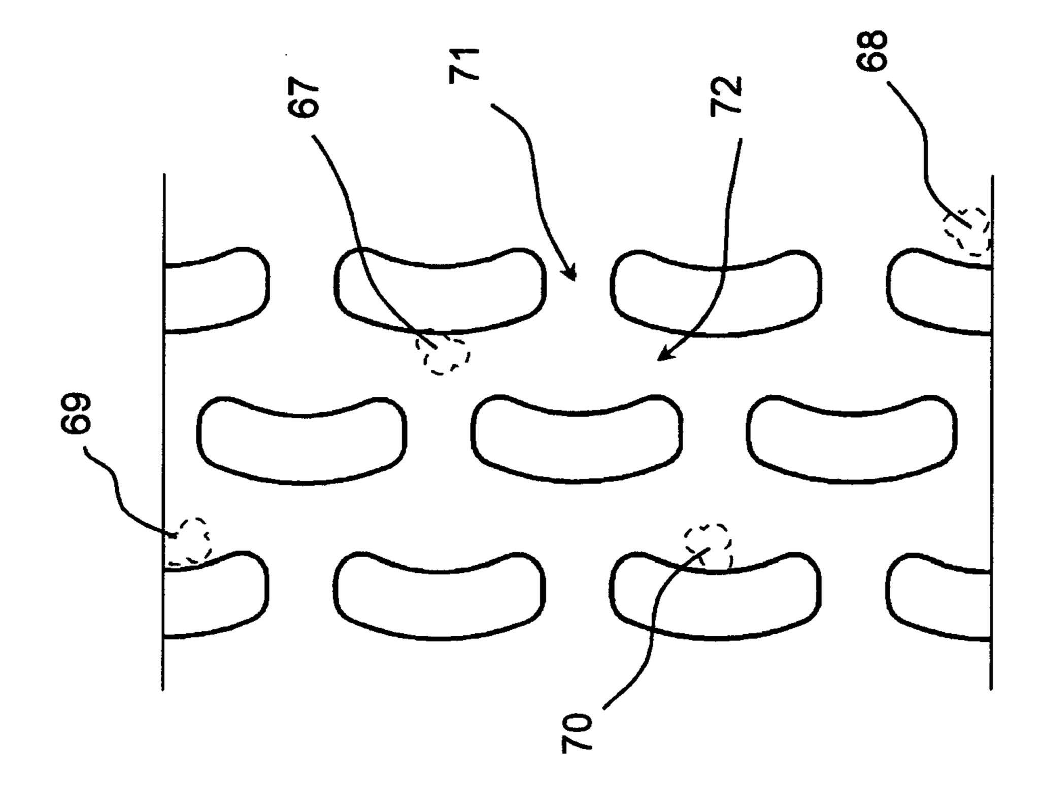
TYPE OF FUEL CELL BIPOLAR PLATES
