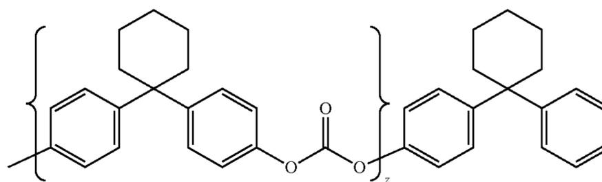
wherein x is an integer between about 40 and about 50 while y and z are integers representing a number of the respective repeating units; a modified bisphenol C polycarbonate
