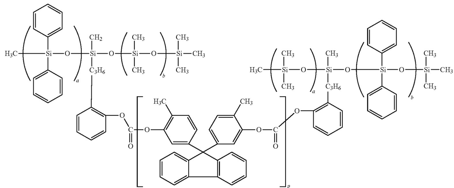
wherein the polymer has an polyalkyl and polyaryl siloxane main chain, and wherein a, b and p are integers representing the number of repeating units;
