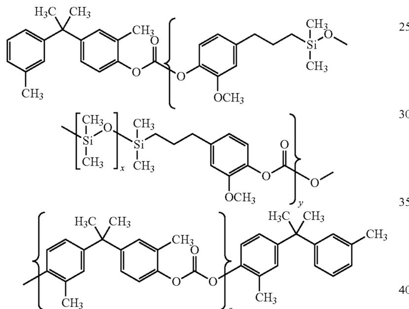
wherein x is an integer between about 40 and about 50 while y and z are integers representing a number of the respective repeating units, a modification of the modified Bisphenol Z polycarbonate of poly(4,4'-diphenyl-1,1'-cyclohexane carbonate) having a small fraction of polydimethyl siloxane in the polymer back bone and having the following formula (IV):
