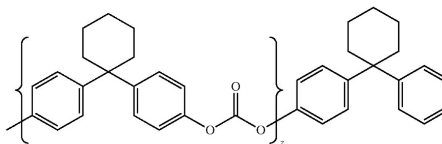
wherein x is an integer between about 40 and about 50 while y and z are integers representing a number of the respective repeating units, a modified Bisphenol C polycarbonate derived from the modification of poly(4,4'-isopropylidene diphenyl carbonate) having a small fraction of polydimethyl siloxane in the polymer backbone and having the following formula (III):
