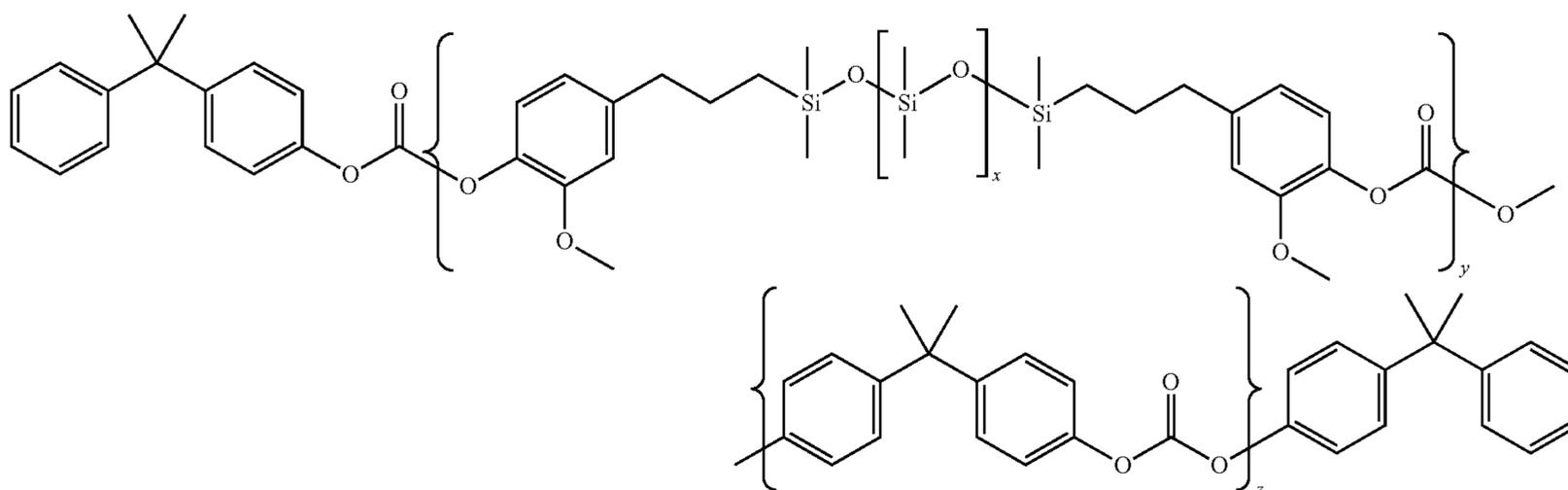
wherein x is an integer between about 40 and about 50 while y and z are integers representing a number of the respective repeating units; a modified bisphenol Z polycarbonate of poly(4,4'-diphenyl-1,1'-cyclohexane carbonate) having a small fraction of polydimethyl siloxane in the polymer back bone and having the following formula (II):
