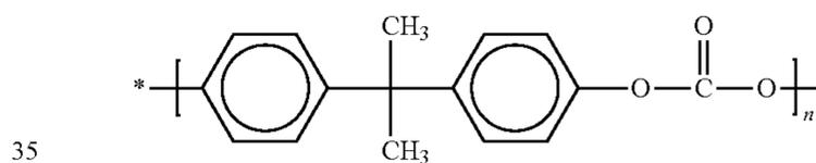
and an extended structure of the bisphenol A polycarbonate is given in below formula (B):
