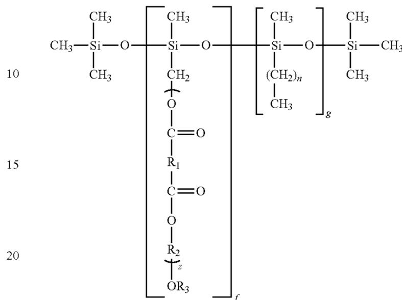
wherein R<sub>1</sub> and R<sub>2</sub> are independently selected from alkylene groups containing from 1 to 10 carbon atoms; R<sub>3</sub> is hydrogen or alkyl having 1 to 3 carbon atoms; n is an
