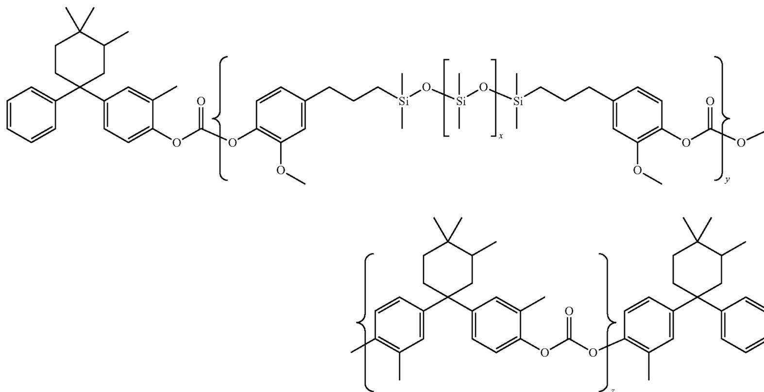
wherein x is an integer between about 40 and about 50 while y and z are integers representing a number of the respective repeating units, and mixtures thereof, and the second low
