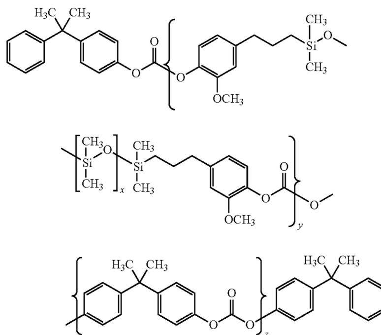
wherein x is an integer between about 40 and about 50 while y and z are integers representing a number of the respective repeating units, a modified Bisphenol Z polycarbonate of poly(4,4'-diphenyl-1,1'-cyclohexane carbonate) having a small fraction of polydimethyl siloxane in the polymer back bone and having the following formula (II):
