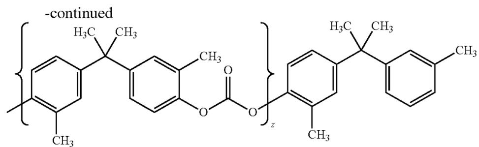
wherein x is an integer between about 40 and about 50 while y and z are integers representing a number of the respective repeating units, a modification of the modified Bisphenol Z polycarbonate of poly(4,4'-diphenyl-1,1'-cyclohexane carbonate) having a small fraction of polydimethyl siloxane in the polymer back bone and having the following formula (IV):
