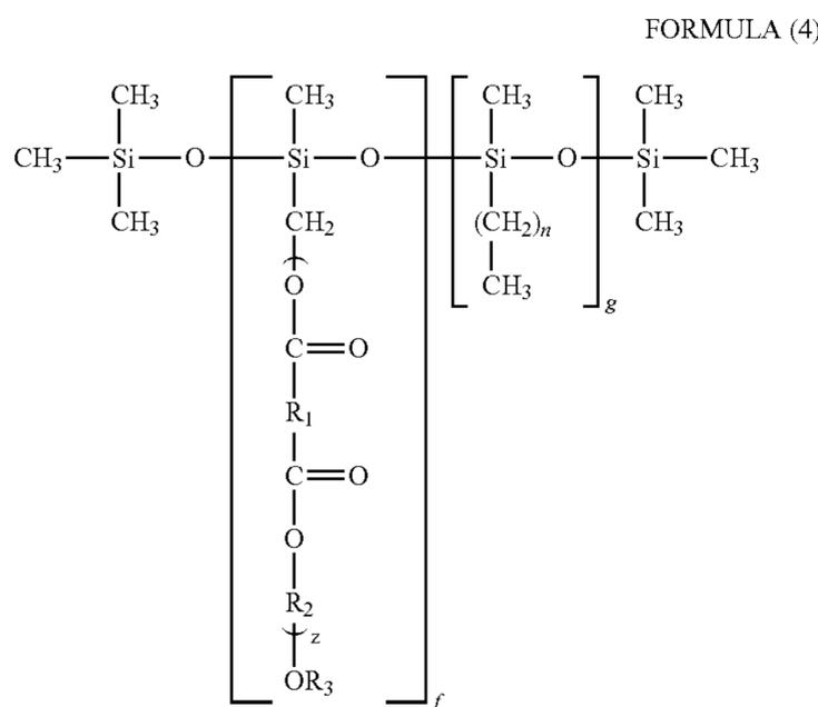
wherein R<sub>1</sub> and R<sub>2</sub> are independently selected from alkylene groups containing from 1 to 10 carbon atoms; R<sub>3</sub> is hydrogen or alkyl having 1 to 3 carbon atoms; n is an integer from 0 to 10; f and g are independently integers from 5 to 500; and z is an integer from 1 to 30. The slip agent lowers the resulting overcoat's surface energy to give slippery surface and render abhesiveness.
