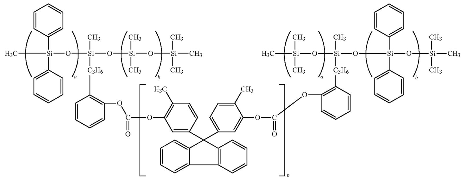
wherein the polymer has an polyalkyl and polyaryl siloxane main chain, and wherein a, b and p are integers representing the number of repeating units;
