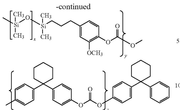
wherein x is an integer between about 40 and about 50 while y and z are integers representing a number of the respective repeating units, a modified Bisphenol C polycarbonate derived from the modification of poly(4,4'-isopropylidene diphenyl carbonate) having a small fraction of polydimethyl siloxane in the polymer back bone and having the following formula (III):
