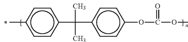
and an extended structure of the bisphenol A polycarbonate is given in below formula (B):
