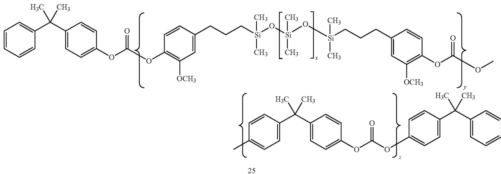
wherein x is an integer between about 40 and about 50 while y and z are integers representing a number of the respective repeating units, a modified Bisphenol Z polycarbonate of poly(4,4'-diphenyl-1,1'-cyclohexane carbonate) having a small fraction of polydimethyl siloxane in the polymer back bone and having the following formula (II):
