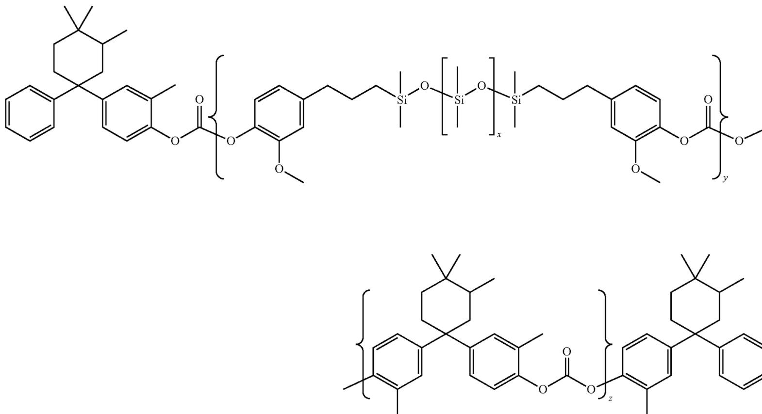
wherein  $x$  is an integer between about 40 and about 50 while  $y$  and  $z$  are integers representing a number of the respective repeating units; and mixtures thereof. The weight average molecular weight of the low surface energy bisphenol type polycarbonates of formulas (I) to (IV) is between about 20,000 and about 200,000.
