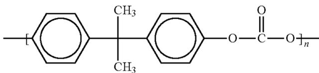
wherein n indicates each respective degree of polymerization, a modified bisphenol A polycarbonate of poly(4,4'-isopropylidene diphenyl)carbonate having the following formula (B):
