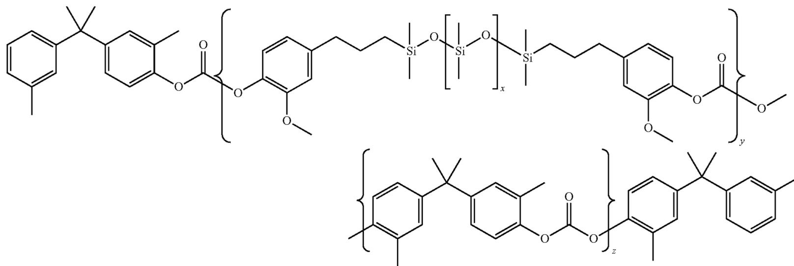
35 wherein x is an integer between about 40 and about 50 while y and z are integers representing a number of the respective repeating units; and a modification of the modified bisphenol Z polycarbonate of poly(4,4'-diphenyl-1,1'-cyclohexane carbonate) having a small fraction of polydimethyl siloxane in the polymer back bone and having the following formula (IV):
