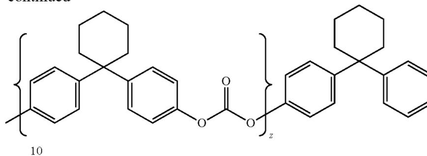
wherein x is an integer between about 40 and about 50 while y and z are integers representing a number of the respective repeating units; a modified bisphenol C polycarbonate derived from the modification of poly(4,4'-isopropylidene
