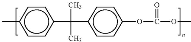
and an extended structure of this bisphenol A polycarbonate is shown in formula (B):
