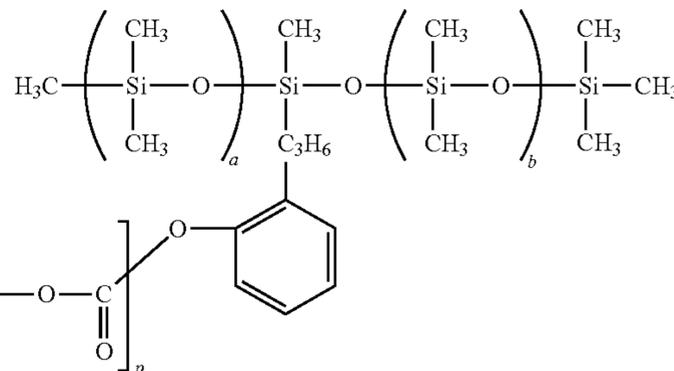
where a, b and p are integers representing the number of repeating units. The weight average molecular weight of the low surface energy polycarbonates of formulas (V) to (XI) is between about 20,000 and about 200,000.
