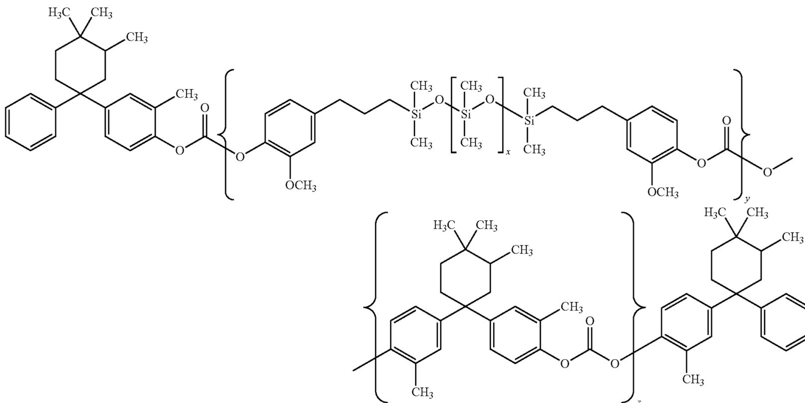
wherein x is an integer between about 40 and about 50 while y and z are integers representing a number of the respective repeating units, and mixtures thereof, and the second low surface energy polymer having a molecular weight of from about 20,000 to about 200,000 is being selected from the group consisting of formula (V):
