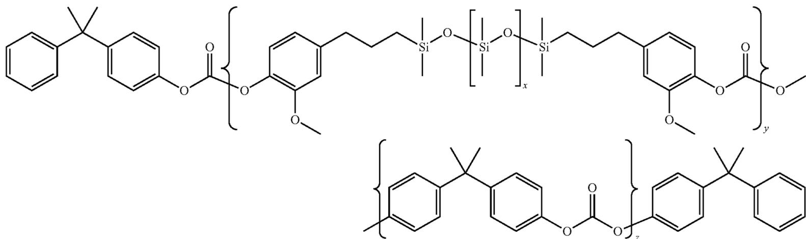
wherein x is an integer between about 40 and about 50 while y and z are integers representing a number of the respective repeating units, a modified Bisphenol Z polycarbonate of poly(4,4'-diphenyl-1,1'-cyclohexane carbonate) having a small fraction of polydimethyl siloxane in the polymer back bone and having the following formula (II):
