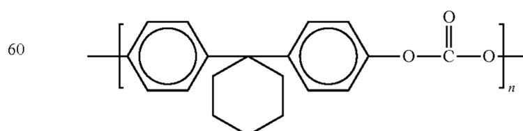
and an extended structure of bisphenol Z polycarbonate is given in formula (D) as follows:
