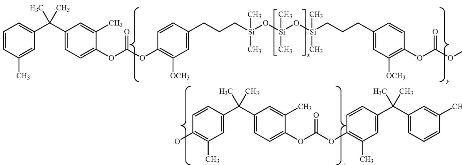
wherein x is an integer between about 40 and about 50 while y and z are integers representing a number of the respective repeating units, a modification of the modified Bisphenol Z polycarbonate of poly(4,4'-diphenyl-1,1'-cyclohexane carbonate) having a small fraction of polydimethyl siloxane in the polymer backbone and having the following formula (IV):
