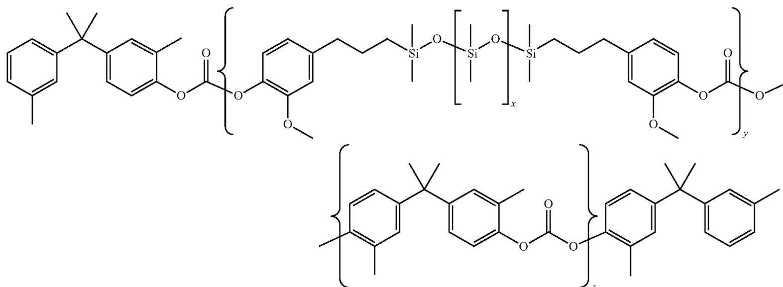
60 wherein x is an integer between about 40 and about 50 while y and z are integers representing a number of the respective repeating units; and a modification of the modified bisphenol Z polycarbonate of poly(4,4'-diphenyl-1,1'-cyclohexane carbonate) of formula (II), having a small fraction of polydimethyl siloxane in the polymer back bone, to give the following
