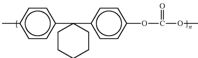
wherein n indicates each respective degree of polymerization, a modified bisphenol Z polycarbonate of poly(4,4'-diphenyl-1,1'-cyclohexane) carbonate having the following formula (D):
