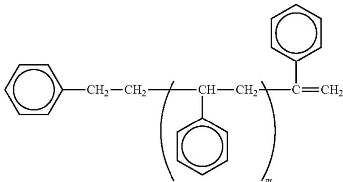
wherein m is the degree of polymerization and m is an integer from about 3 to about 10.
