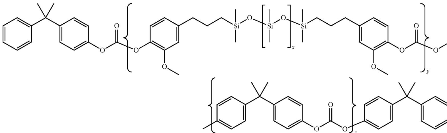
wherein x is an integer between about 40 and about 50 while y and z are integers representing a number of the respective repeating units, a modified Bisphenol Z polycarbonate of
