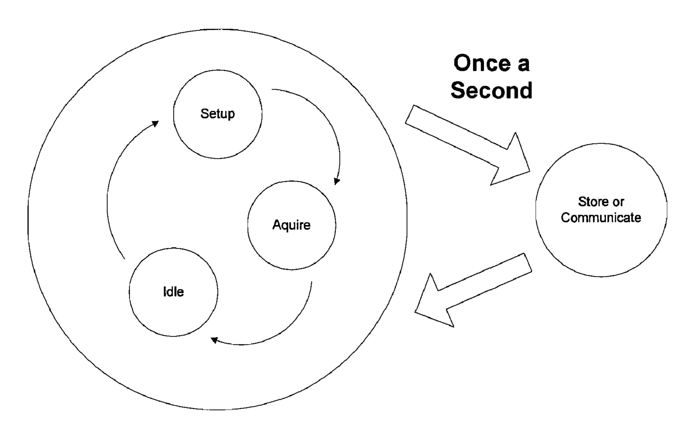
Continuous Loop based on Sample Rate
