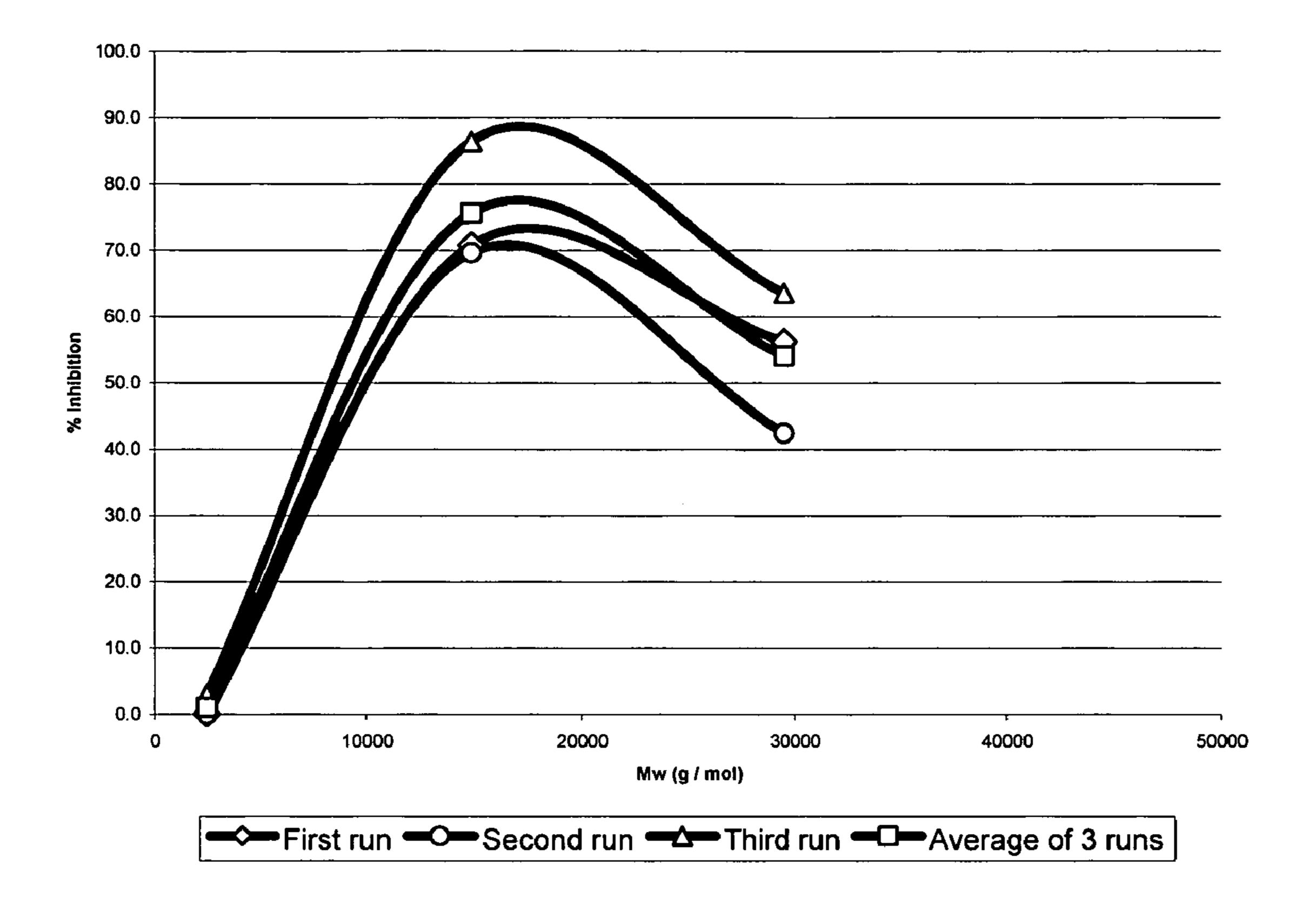
% Inhibition of calcium carbonate vs. Mw of guar 1.6 DS at 10ppm active
