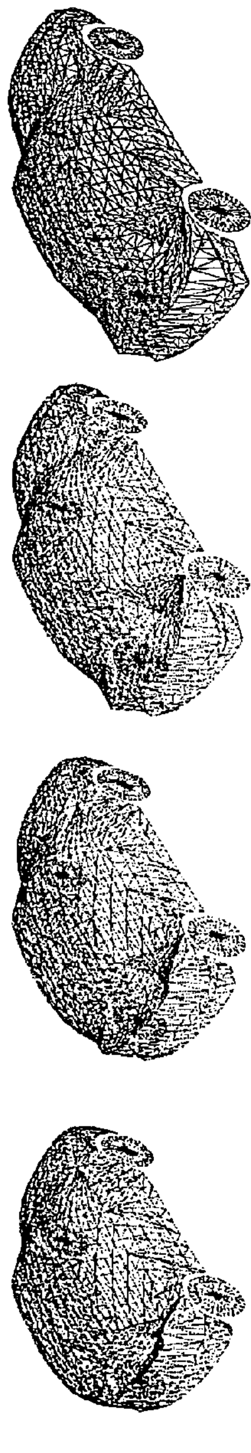
(a) The mesh ASM model morphing: from a hatchback to a sedan
