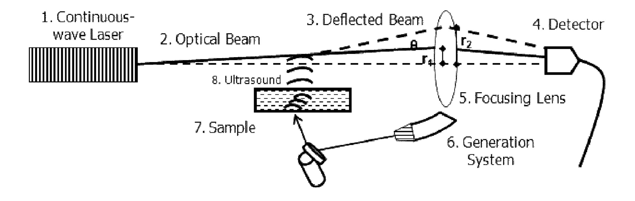
Figure 3: Arrangement for the sensing of ultrasound created by a CLGU 6 using Gas-coupled laser acoustic detection. Ultrasonic waveforms 8, upon transmission through the material 7, radiate an airborne wave. This modulates the index of refraction transverse to the probe beam 2 and causes a change in the direction of the optical beam path 3. The change is detected by a position-sensitive photodetector 4.
