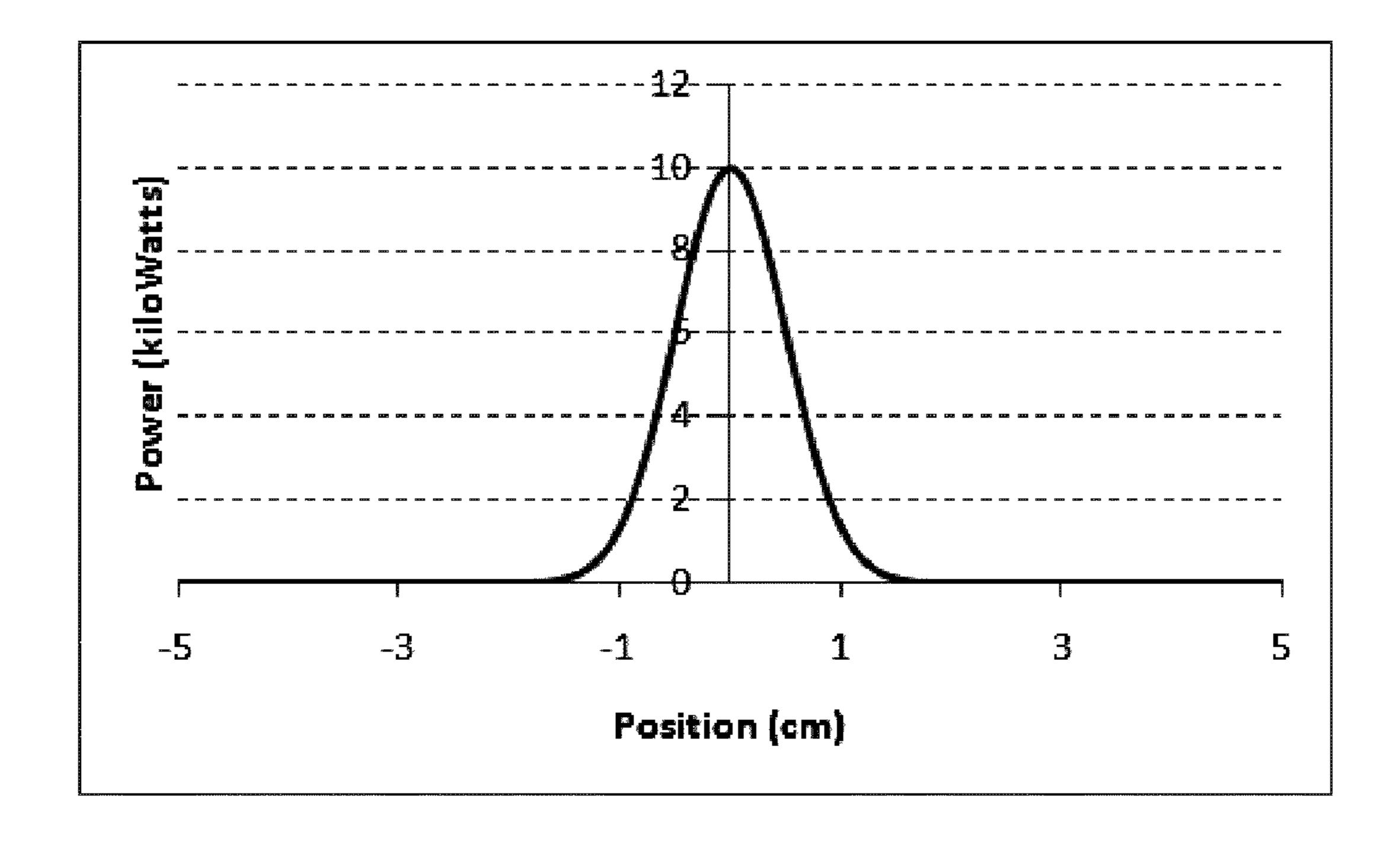
Figure 4: A Gaussian profile that simulates the power distribution of a ideal continuous laser. The x-axis is in centimeters and the y-axis shows the power. This beam would have a width at half the maximum value of about 2 centimeters.
