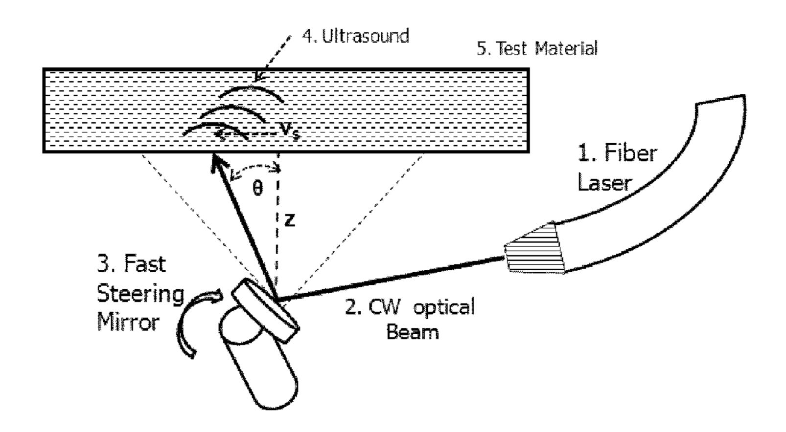
Conceptual drawing for the implementation of Continuous Laser Generation of Ultrasound. The optical beam 2 from a high-power continuous laser 1 is directed to a scanning mirror 3. The mirror rotates, controlled electronically, sweeping the beam along a line across the sample 5. This action creates ultrasound 4 in the material that can be used for nondestructive evaluation of the material properties.
