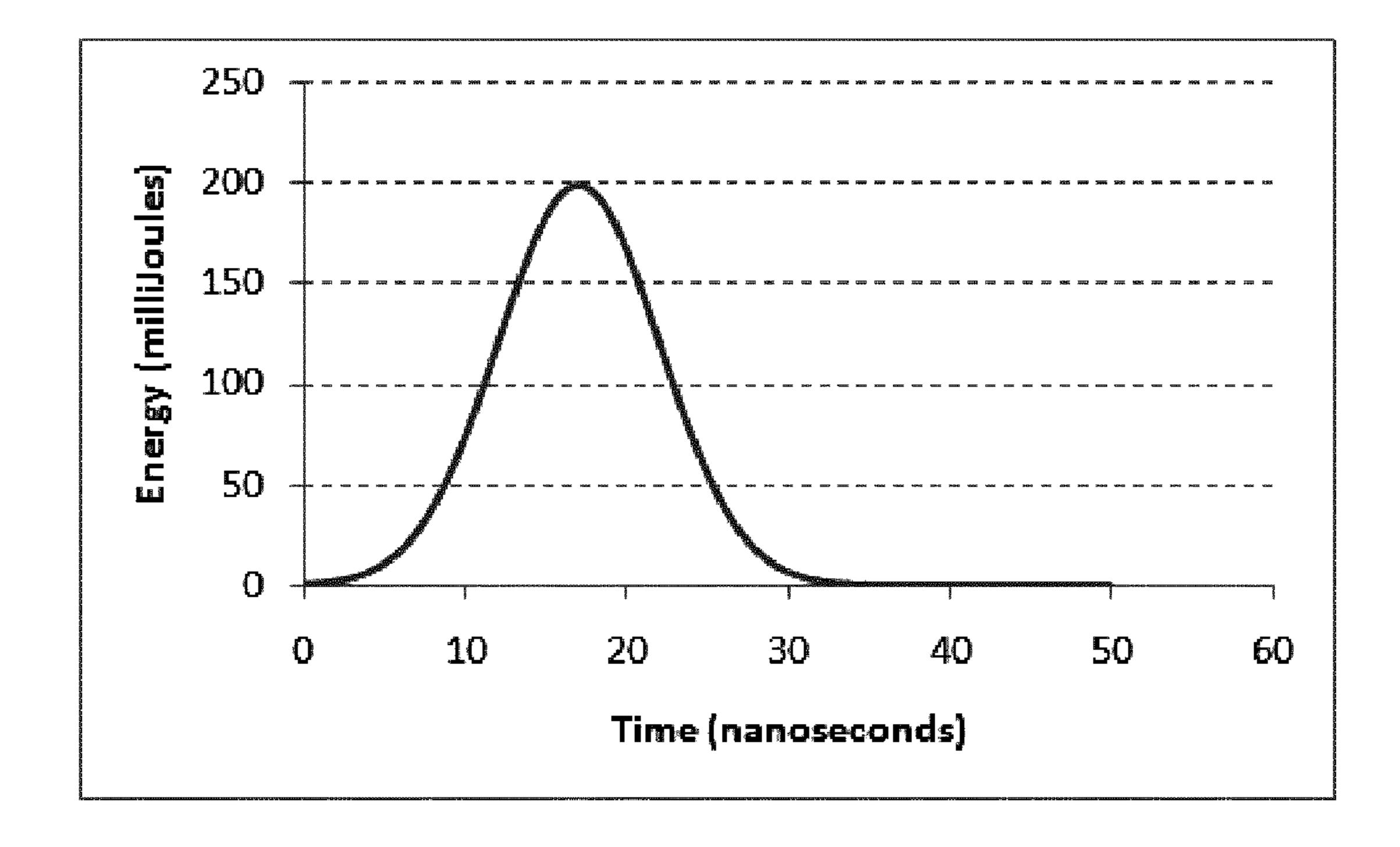
Figure 2: A Gaussian distribution curve that is used to simulate the time profile of a laser pulse. The x-axis is time in nanoseconds whereas the y-axis is energy. The pulse has a width at half the maximum value of 15 nanoseconds.
