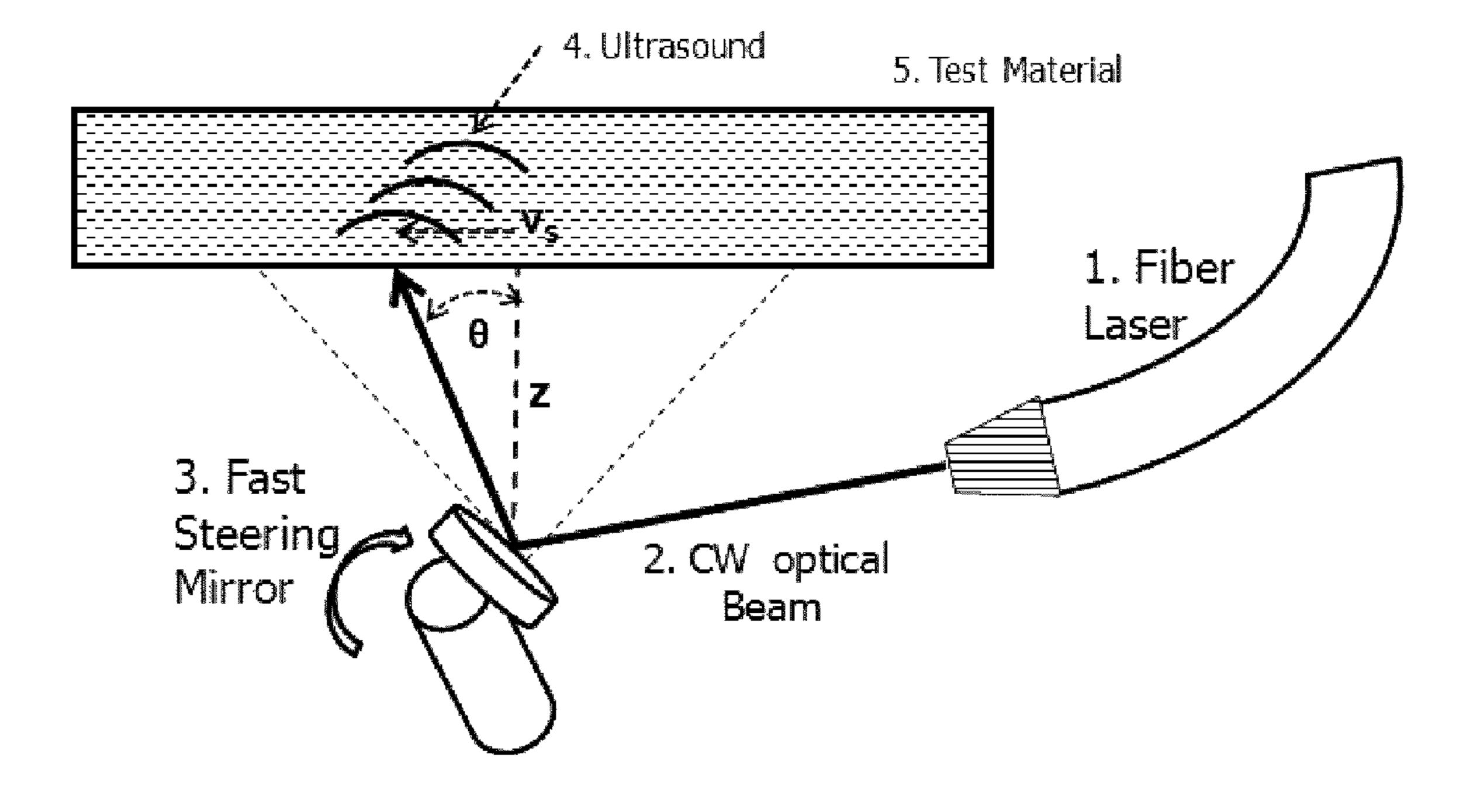
Figure 1: Conceptual drawing for the implementation of Continuous Laser Generation of Ultrasound. The optical beam 2 from a high-power continuous laser 1 is directed to a scanning mirror 3. The mirror rotates, controlled electronically, sweeping the beam along a line across the sample 5. This action creates ultrasound 4 in the material that can be used for nondestructive evaluation of the material properties.
