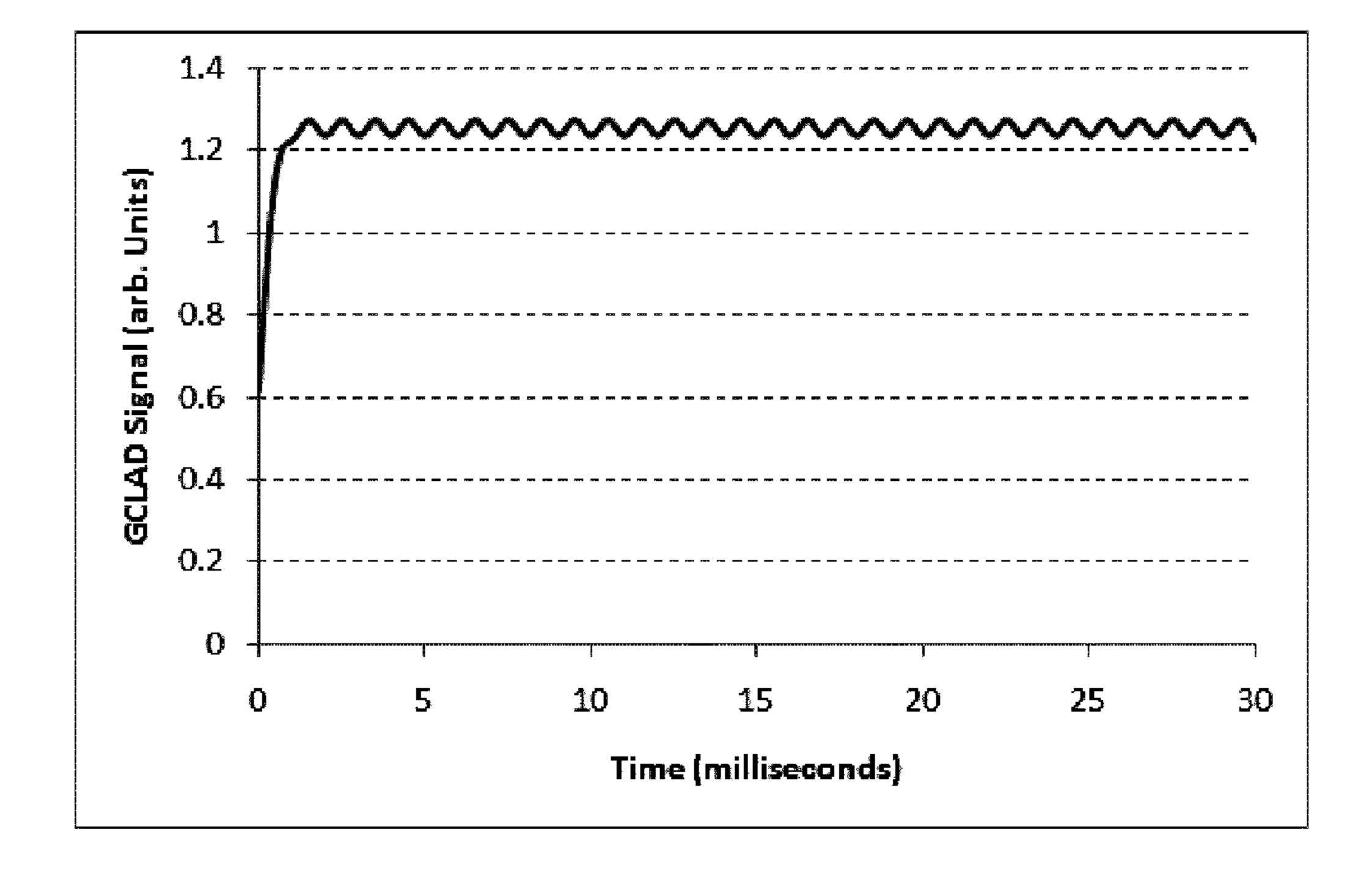
Figure 5: When the material is swept by the laser, each point gives rise to a Gaussian-type curve. The summation of all curves as a function of time simulates the signal received by a GCLAD detection system. This graph was created using Equation 4 and the laser profile of Figure 3. It is essentially the sum of 30 waveforms separated by 1 ms each.
