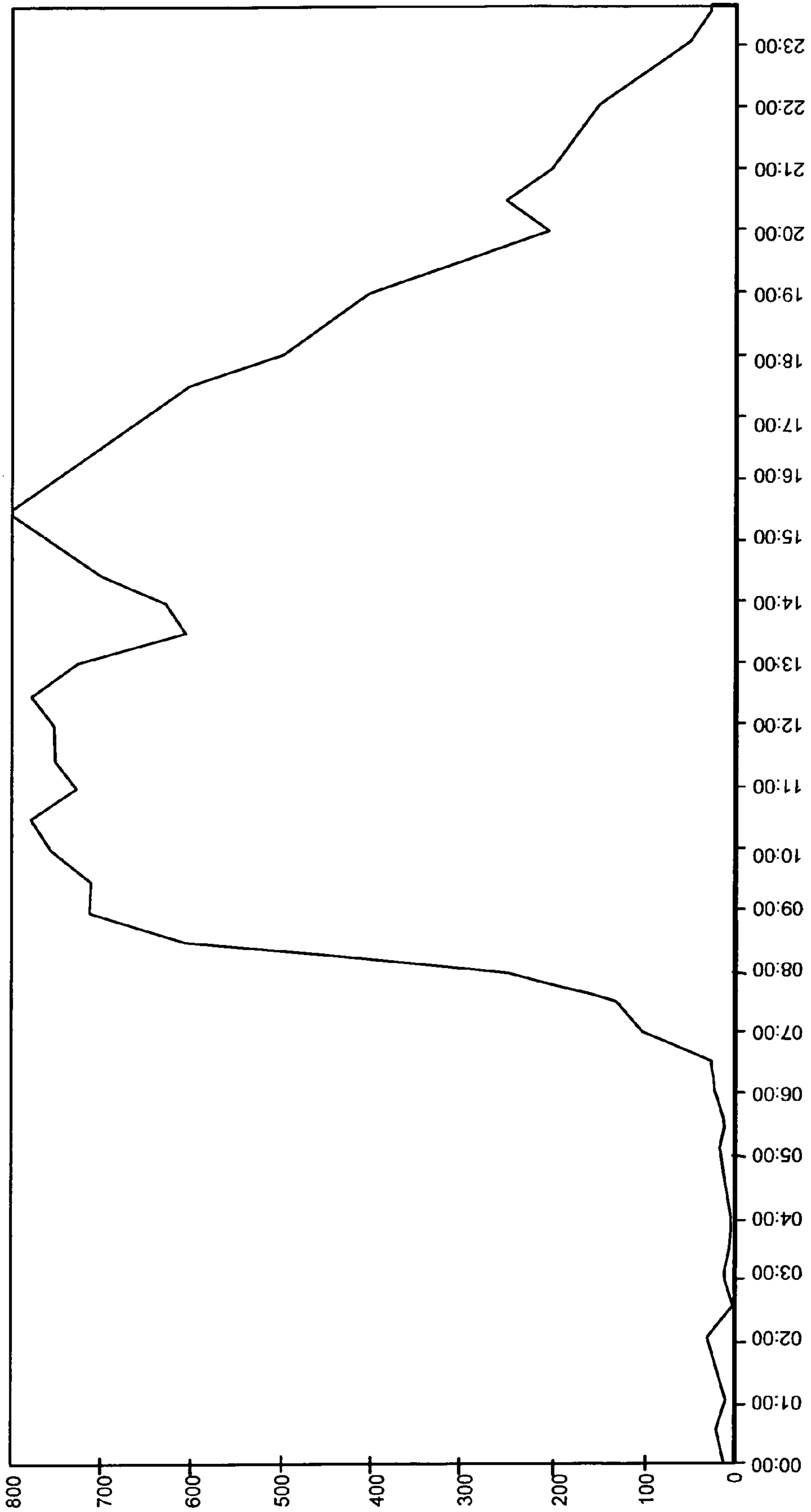
Typical 24 Hour Radio Site Loading
