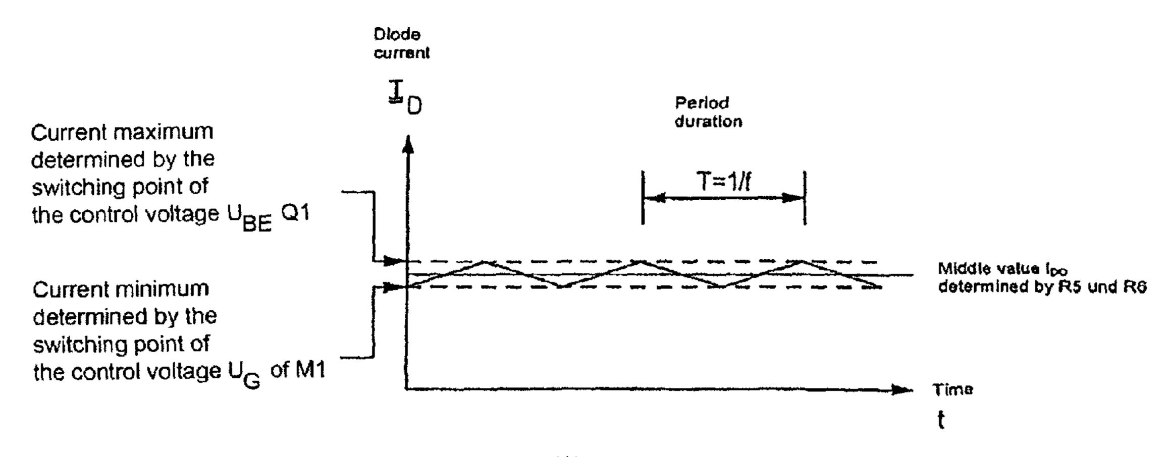
Frequency: f < 100 kHz (determined by Unerz and suitable dimensioning of L1 and the switching thresholds for the control voltages Use and Uo of the power transistors Q1 and M1)
