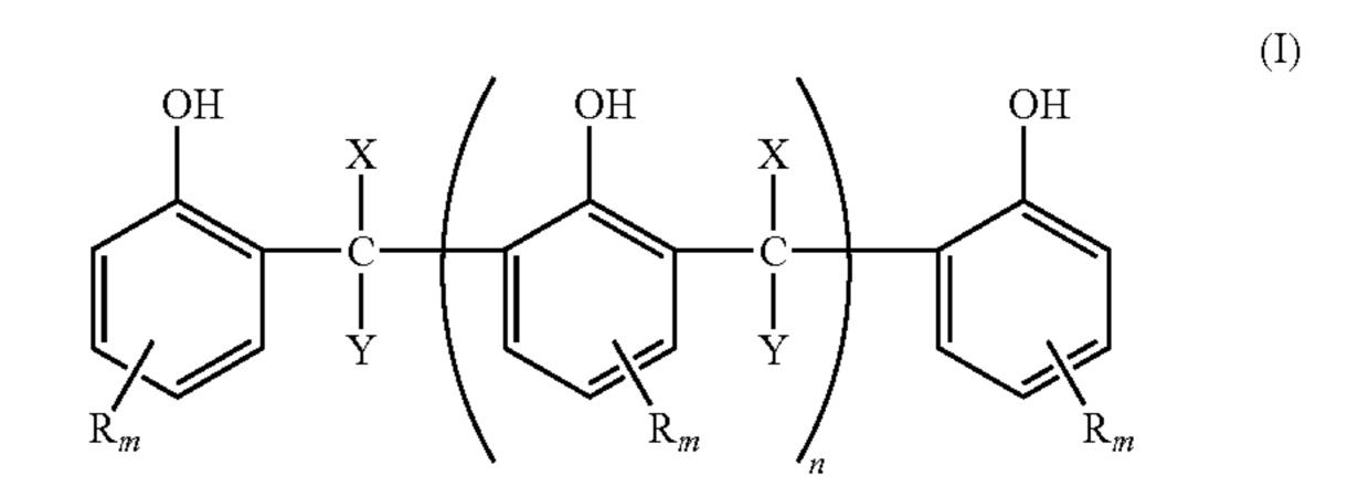
wherein R is a hydrogen atom, a halogen atom, a hydroxyl group, a lower alkyl group, an alkoxyl group, a cyano group, a nitro group, an aryl group or an aralkyl group, R in the number of m may be the same or different, m is an integer of 0 to 3, n is an integer of 0 to 3, and X and Y are each a hydrogen atom, an alkyl group or an aryl group.
