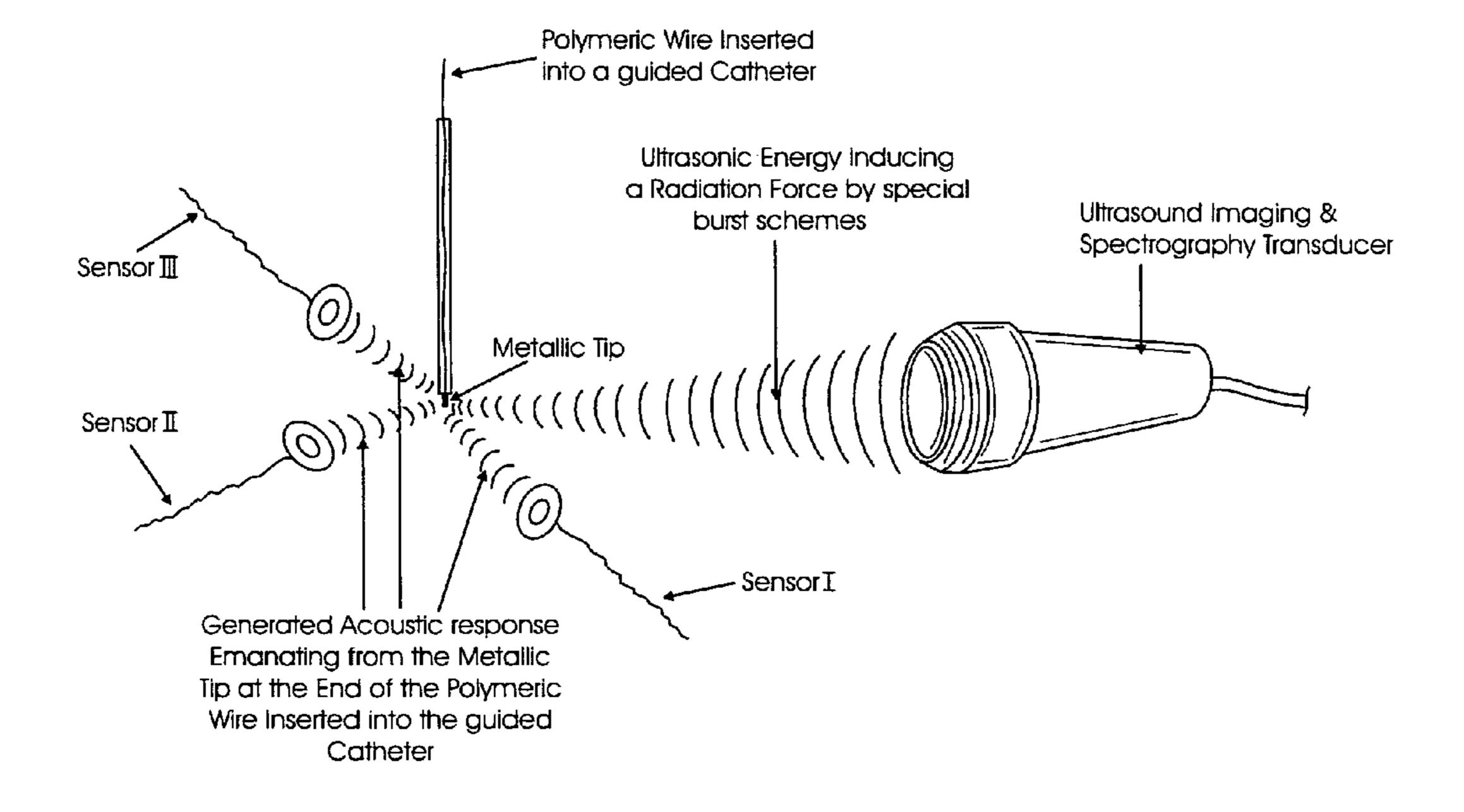
Figure 1: Schematic presentation of the present invention of IDUS for intrabody catheter positioning
