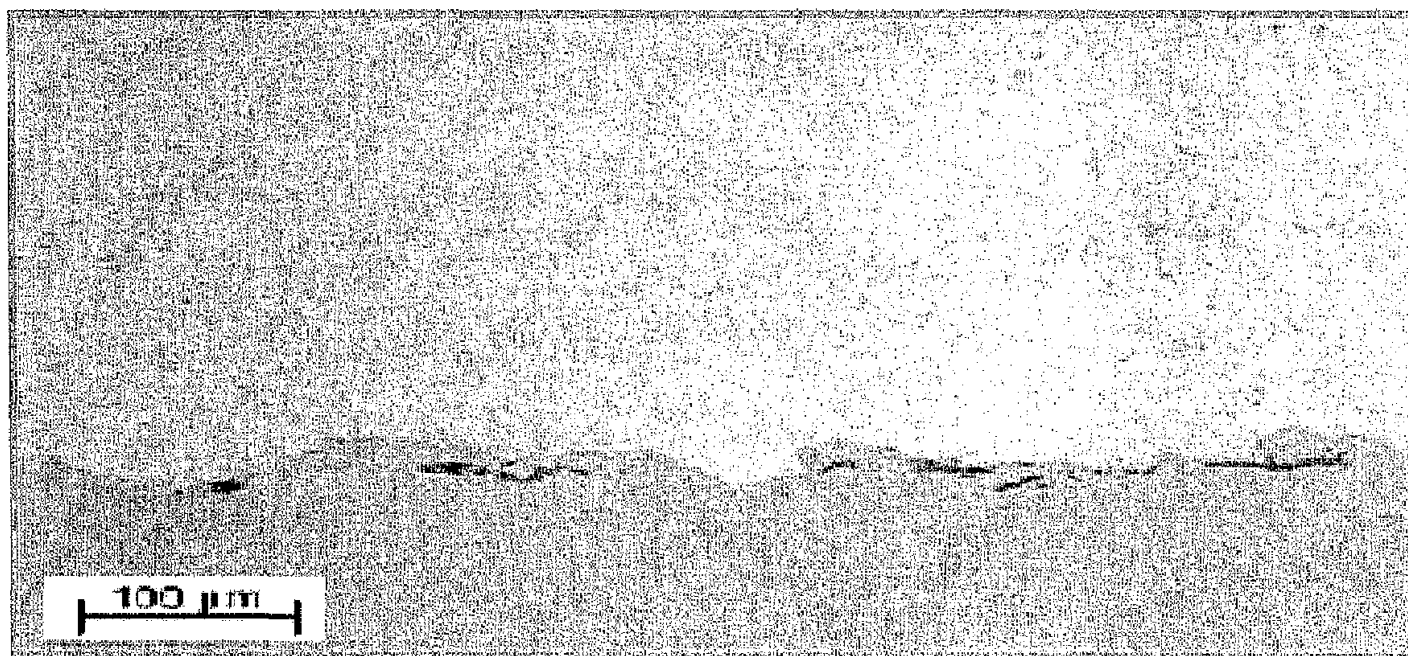
FIGURE 26 B The Cu has a flattened structure
