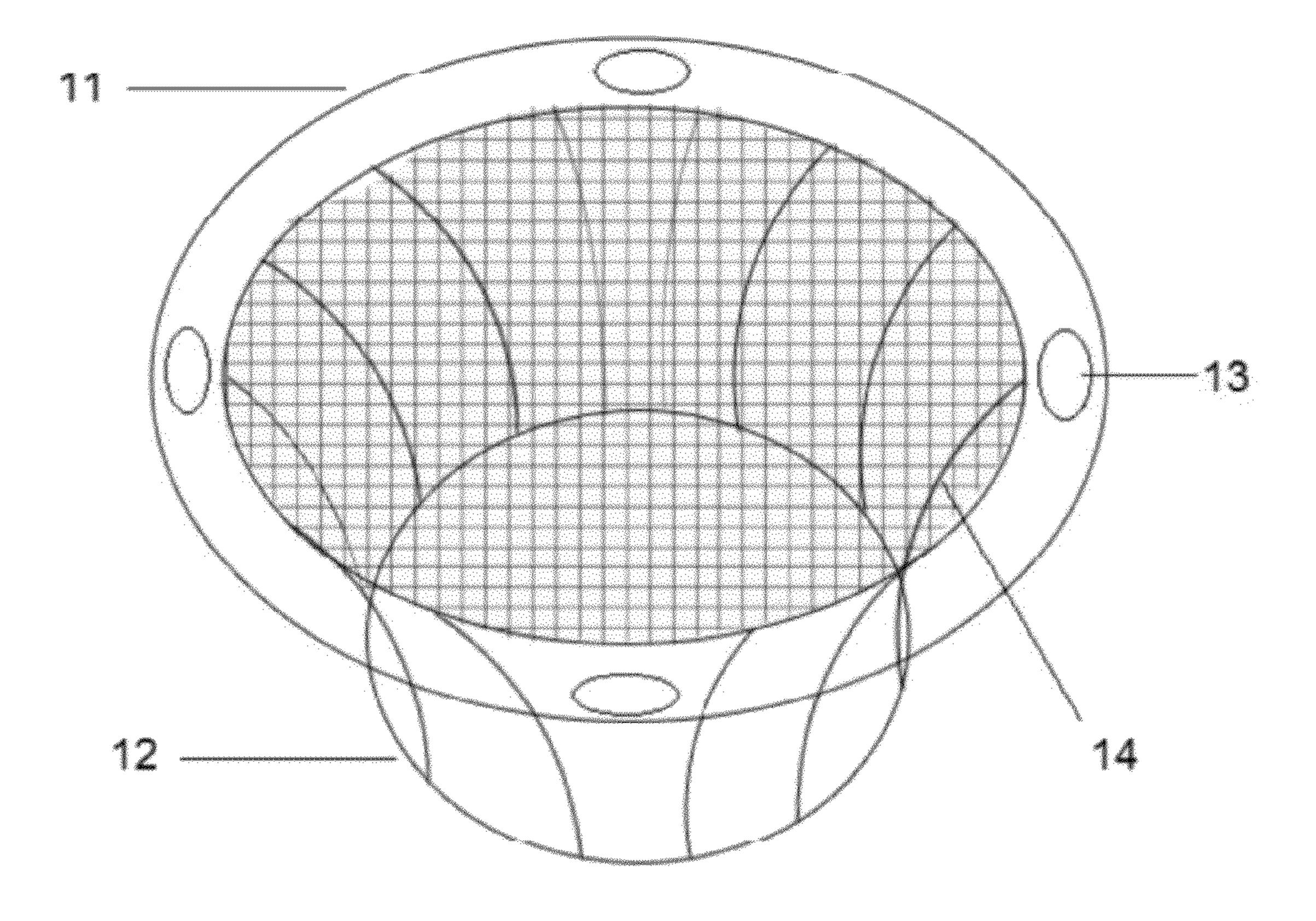
Figure 3. A Seal-Fixation Adaptor
