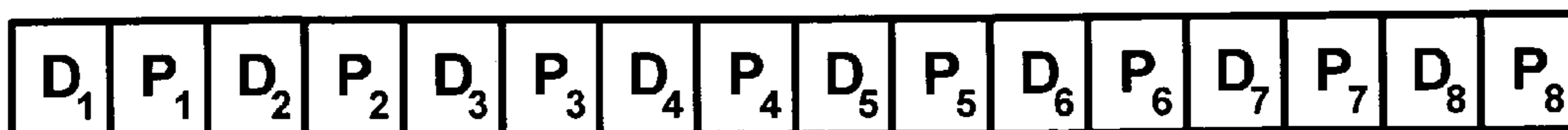
Fig. 19 Bit Order for SCCC M/H Transmissions
