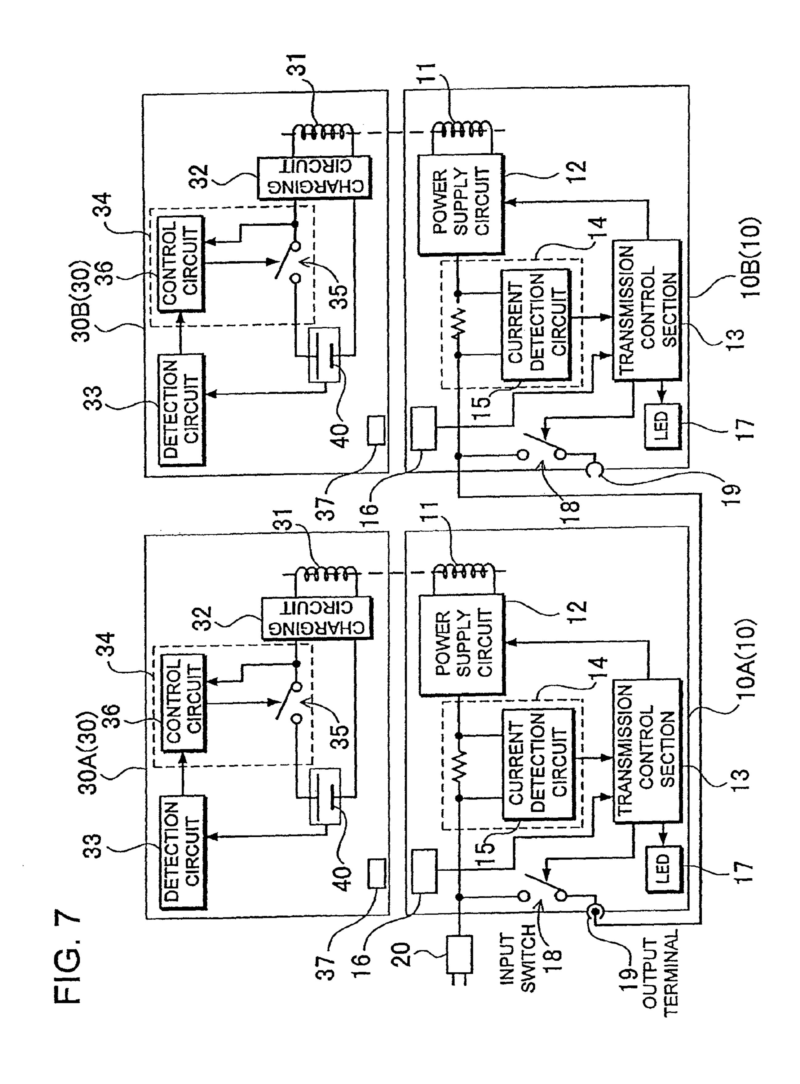
METHOD OF DATA TRANSMISSION EMBEDDED IN ELECTRIC POWER TRANSMISSION AND A CHARGING STAND AND BATTERY DEVICE USING TRANSMITTING COIL CURRENT CHANGE TO RECEIVE THAT DATA TRANSMISSION
