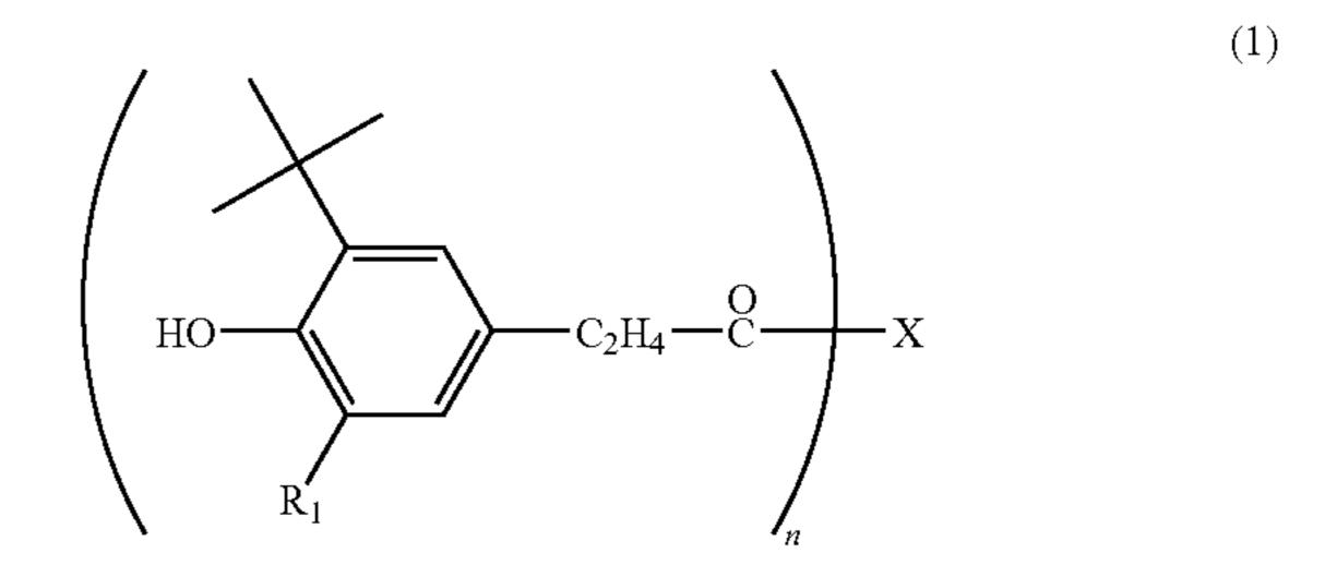
wherein R<sub>1</sub> is an alkyl group having 1 to 8 carbon atoms, X is an n-valent alcohol residue having 1 to 18 carbon atoms optionally containing a heteroatom, a cyclic group, or a heteroatom and a cyclic group, and n is an integer of 1 to 4, and not less than 20 parts by weight and not more than 50 parts by weight of a binder to obtain a granular agglomerate; and
