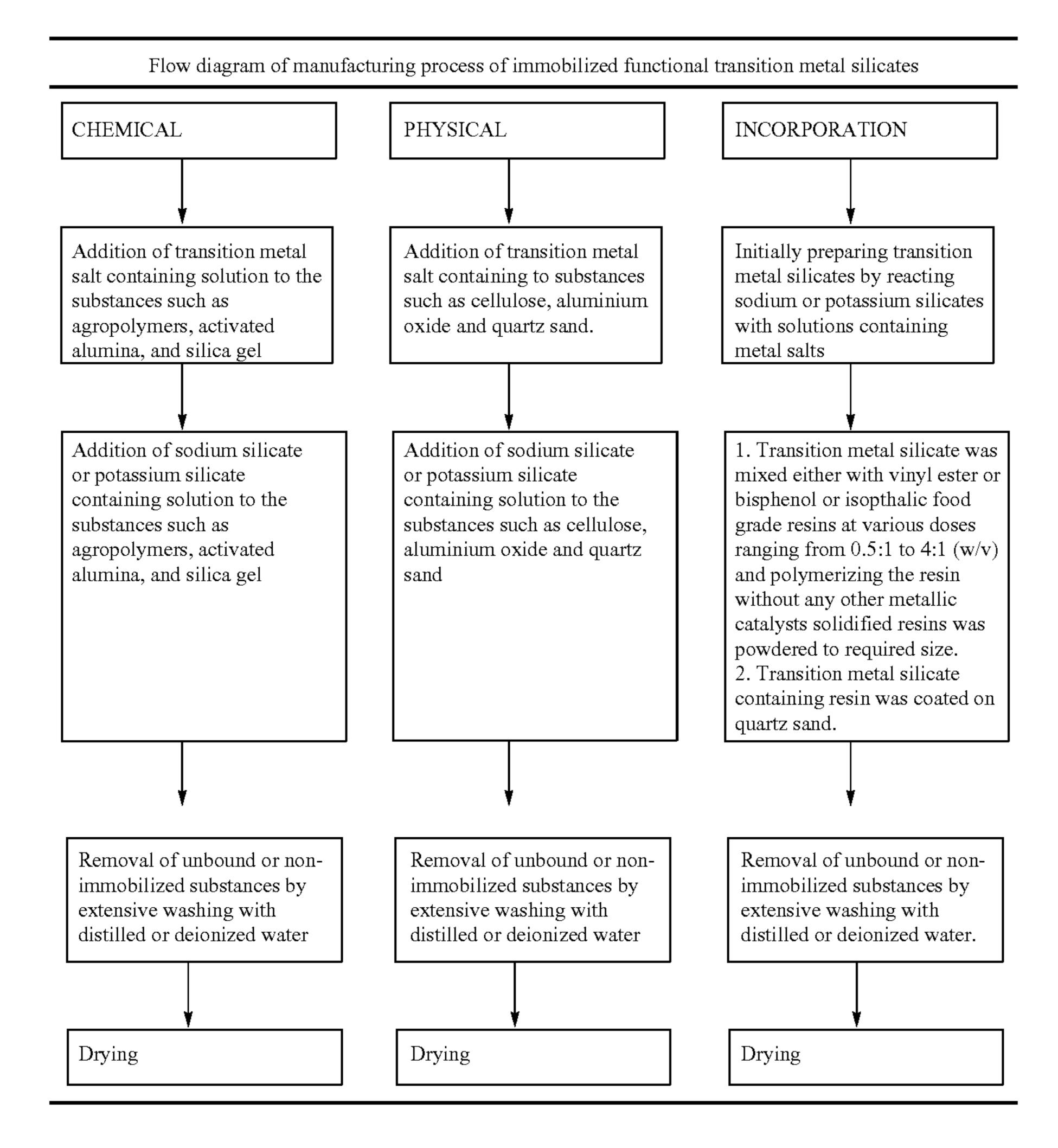
In the embodiment of present invention, a method of 40 decontamination of toxic metals, like arsenic, mercury etc., and disinfection of microbes such as fungi, bacteria, viruses, and protozoa by functional transition metal silicates is described.
