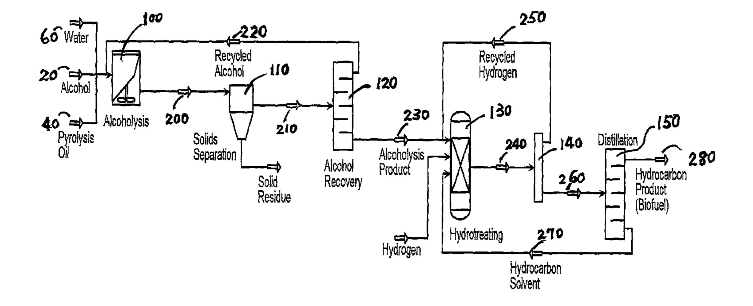
oil alcoholysis with subsequent hydrotreating Schematic representation of the steps involved in pyrolysis
