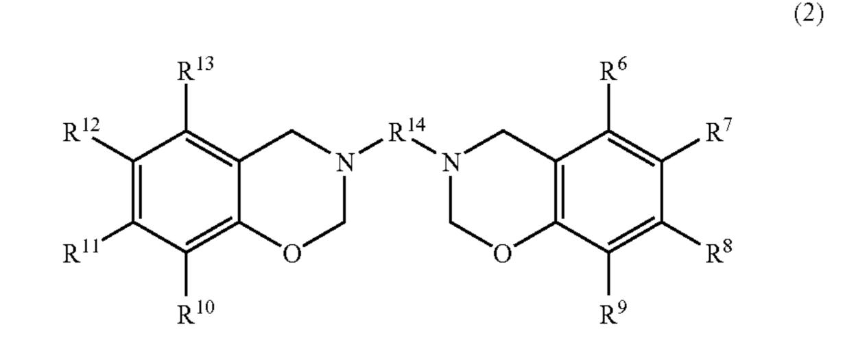
where, R<sup>6</sup> to R<sup>13</sup> represent a hydrogen atom, an alkyl group, or the like, and R<sup>14</sup> represents a divalent saturated alicyclic hydrocarbon group having a condensed ring structure.
