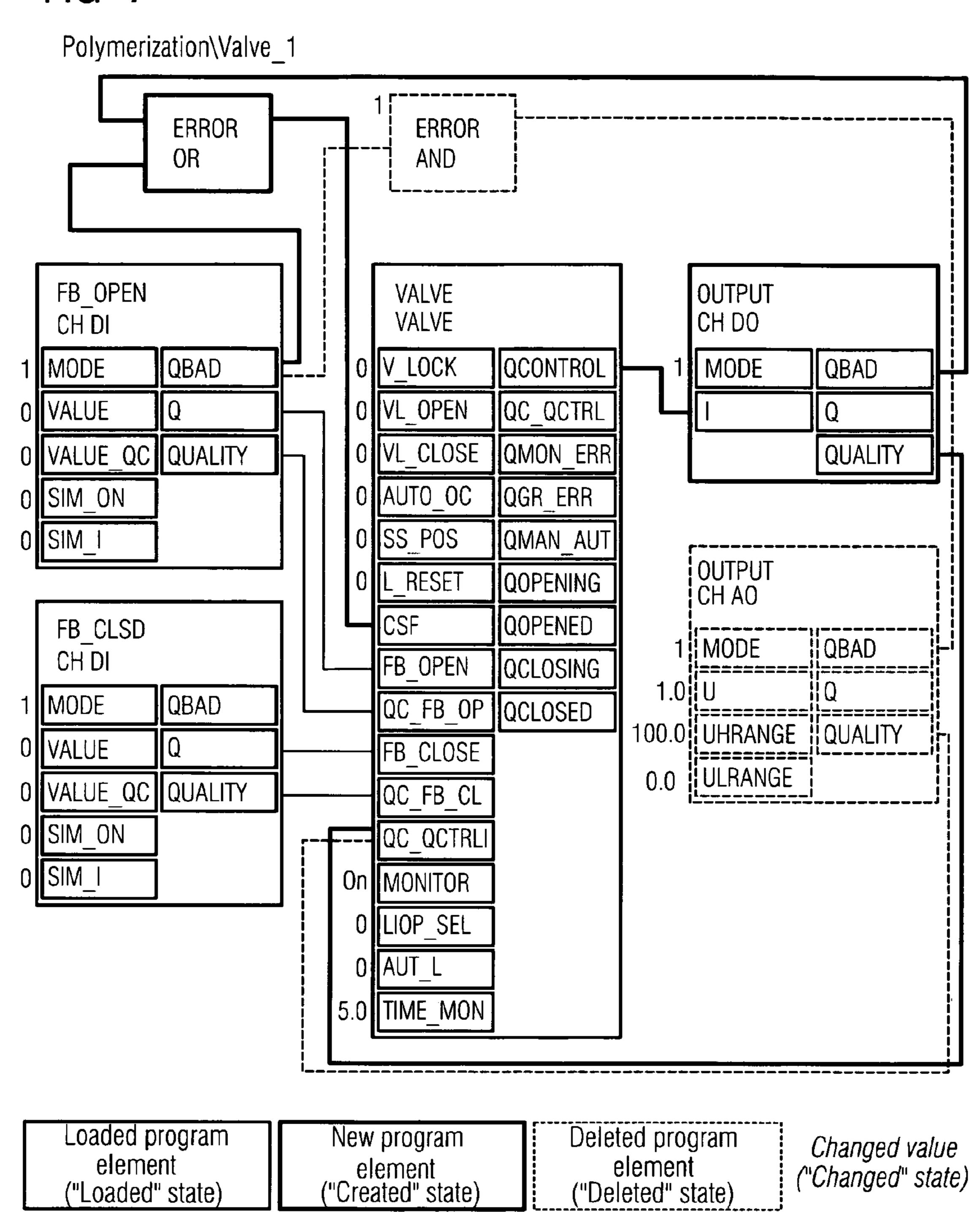
The new OR function with the name ERROR has been inserted into the source plan VALVE\_1. The AND function with the name ERROR on the other hand has been deleted, but is still present in the controller memory.
