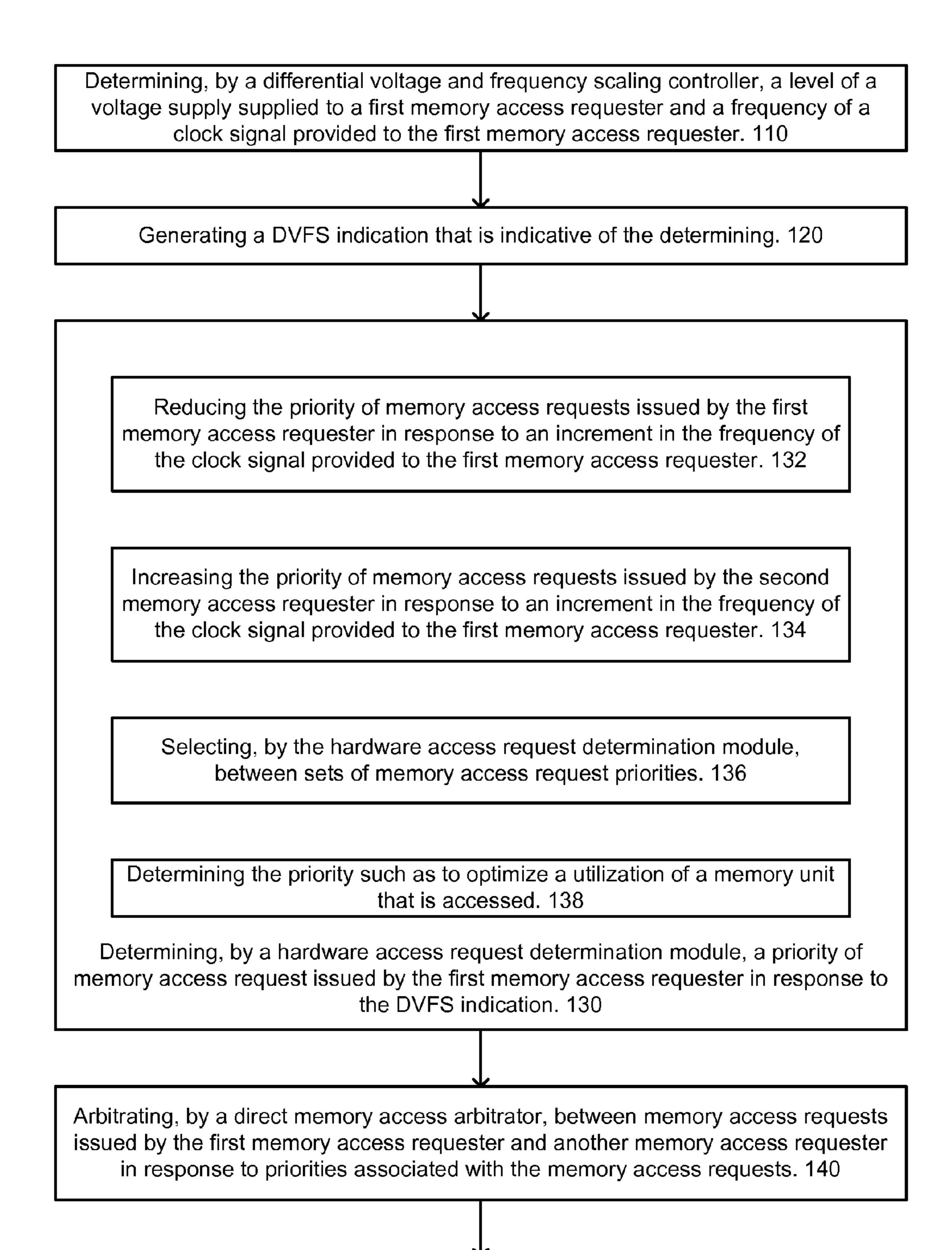
Accessing the memory unit according to the memory access request that won the arbitration. 150
