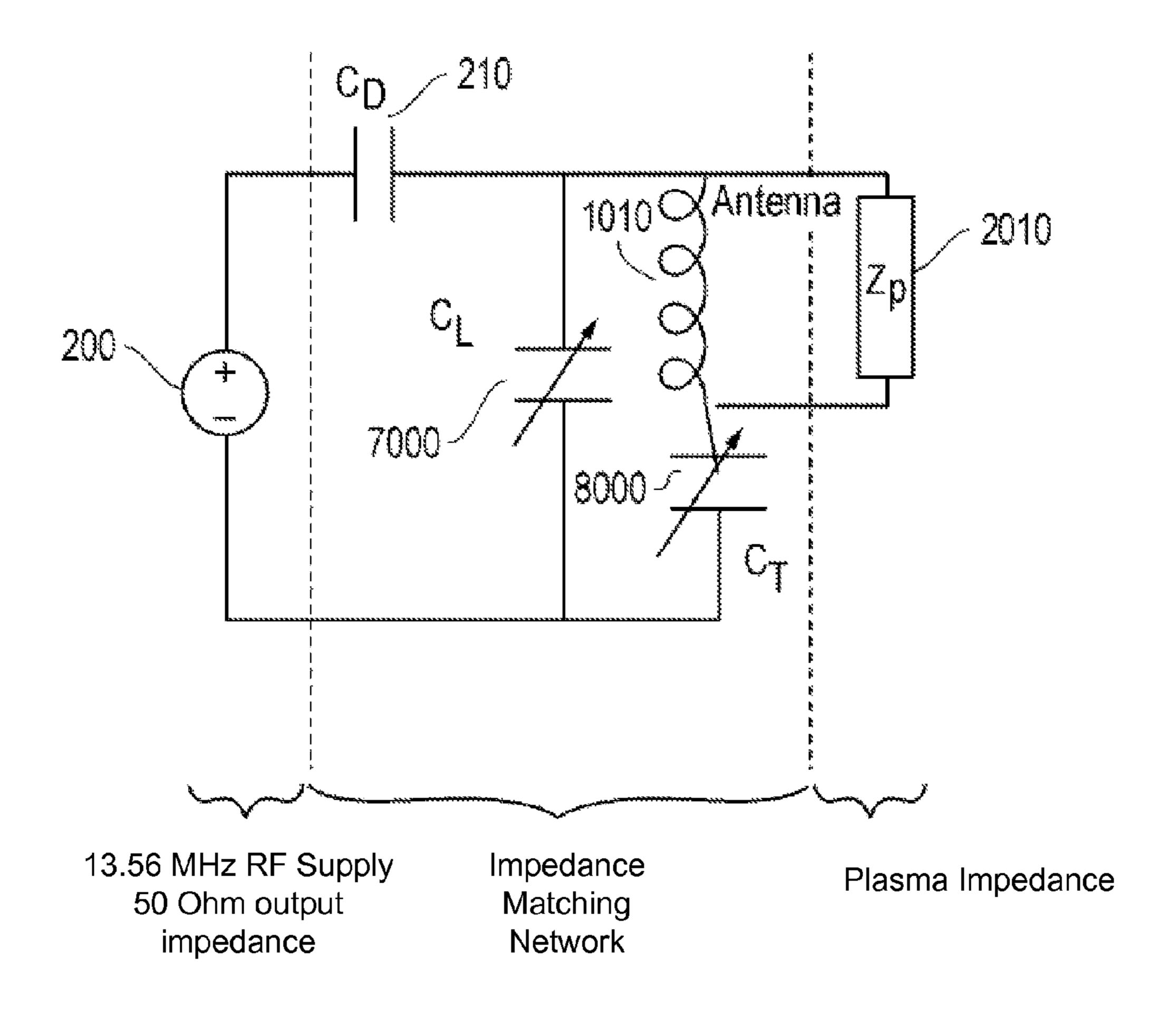
$C_D$ =200pF,  $C_L$ =92pF, $C_T$ =216pf, Phase shift across antenna  $\cong$ 0°  $C_D$ =50pF,  $C_L$ =330pF, $C_T$ =340pf, Phase shift across antenna  $\cong$ 180°
