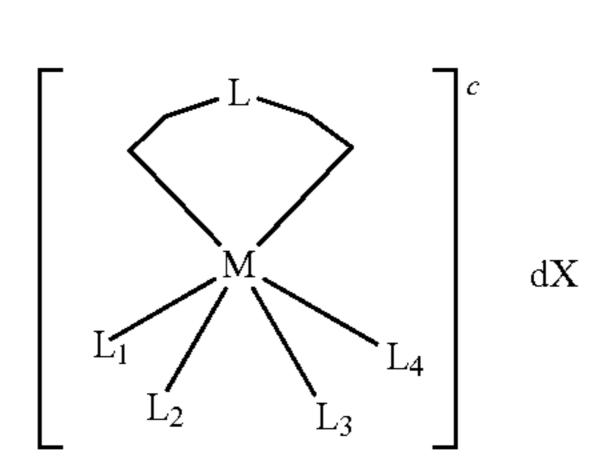
M is a transition metal and is typically iron, cobalt, ruthenium, osmium, or vanadium. Ruthenium and osmium are particularly suitable for redox mediators.
