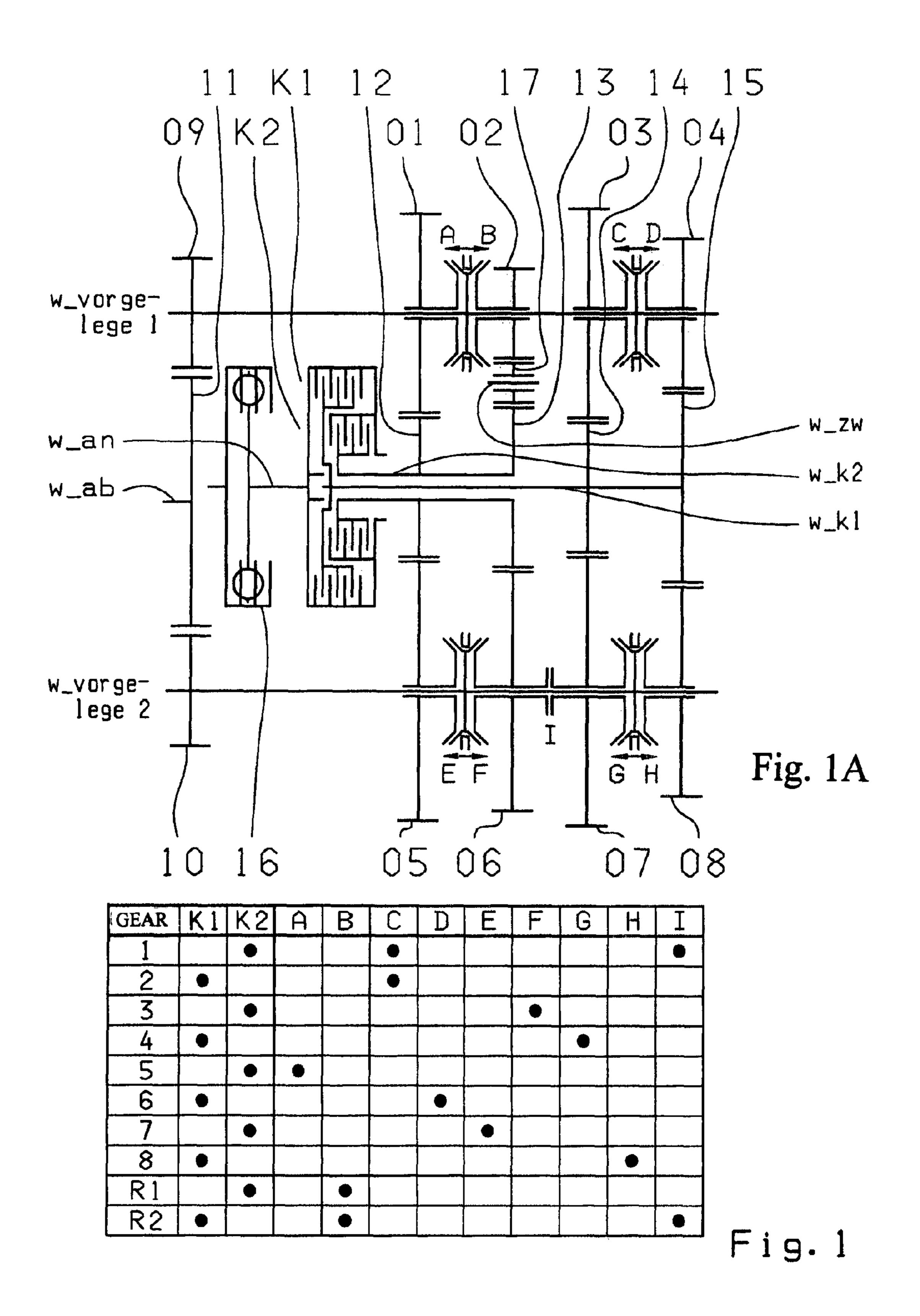
fewest possible wheel planes, preferably such that all the forward gears and reverse gears can be shifted under load in sequence.
