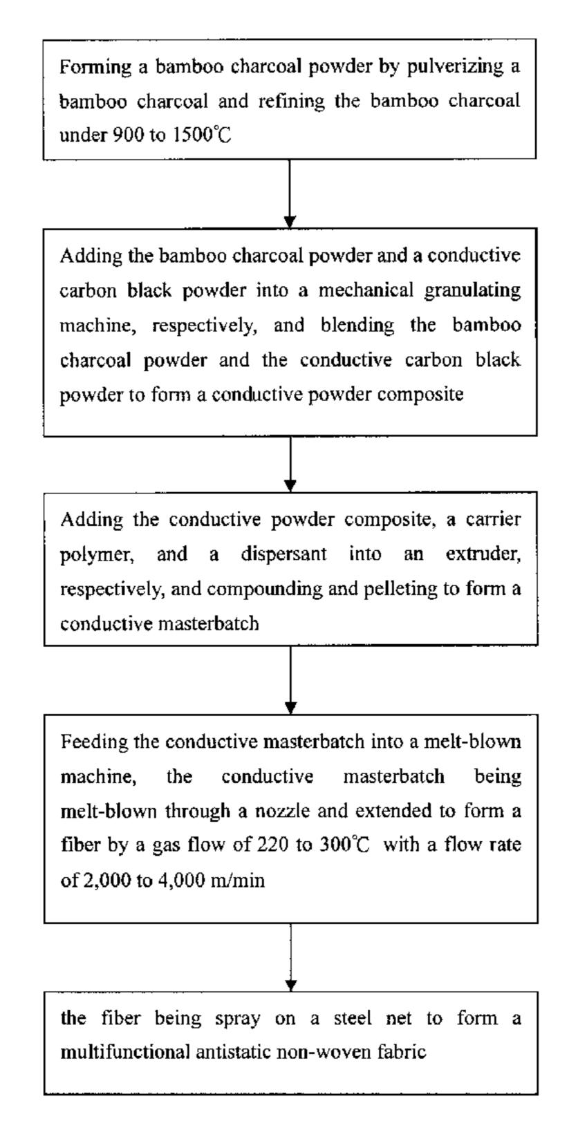
Forming a bamboo charcoal powder by pulverizing a bamboo charcoal and refining the bamboo charcoal under 900 to 1500°C
