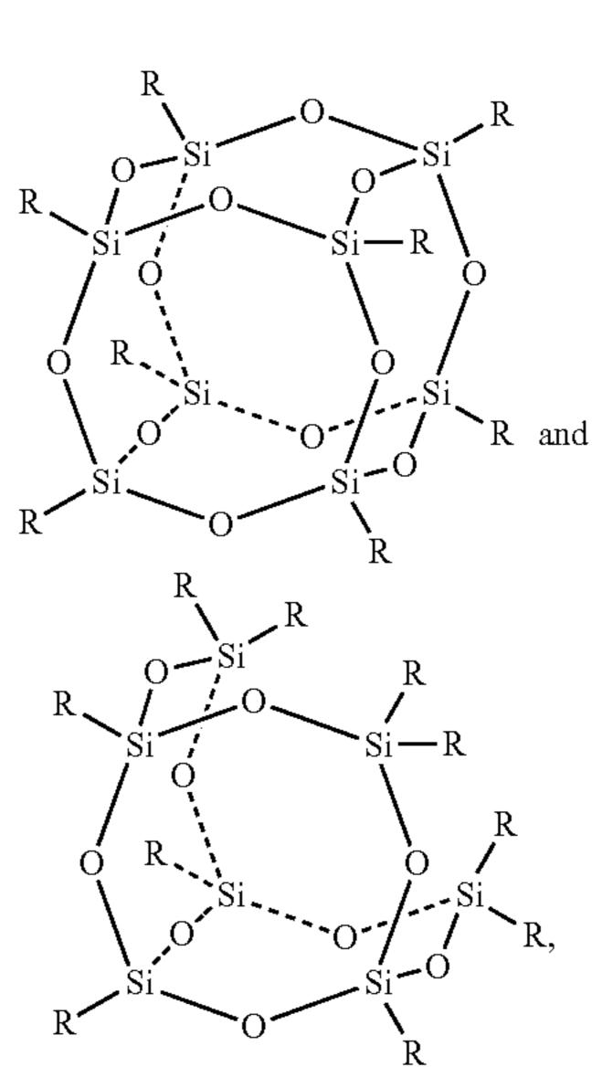
wherein R is one or more substituent groups, at least one of which is capable of forming a chemical bond between polyhedral oligomeric silsesquioxane molecules.
