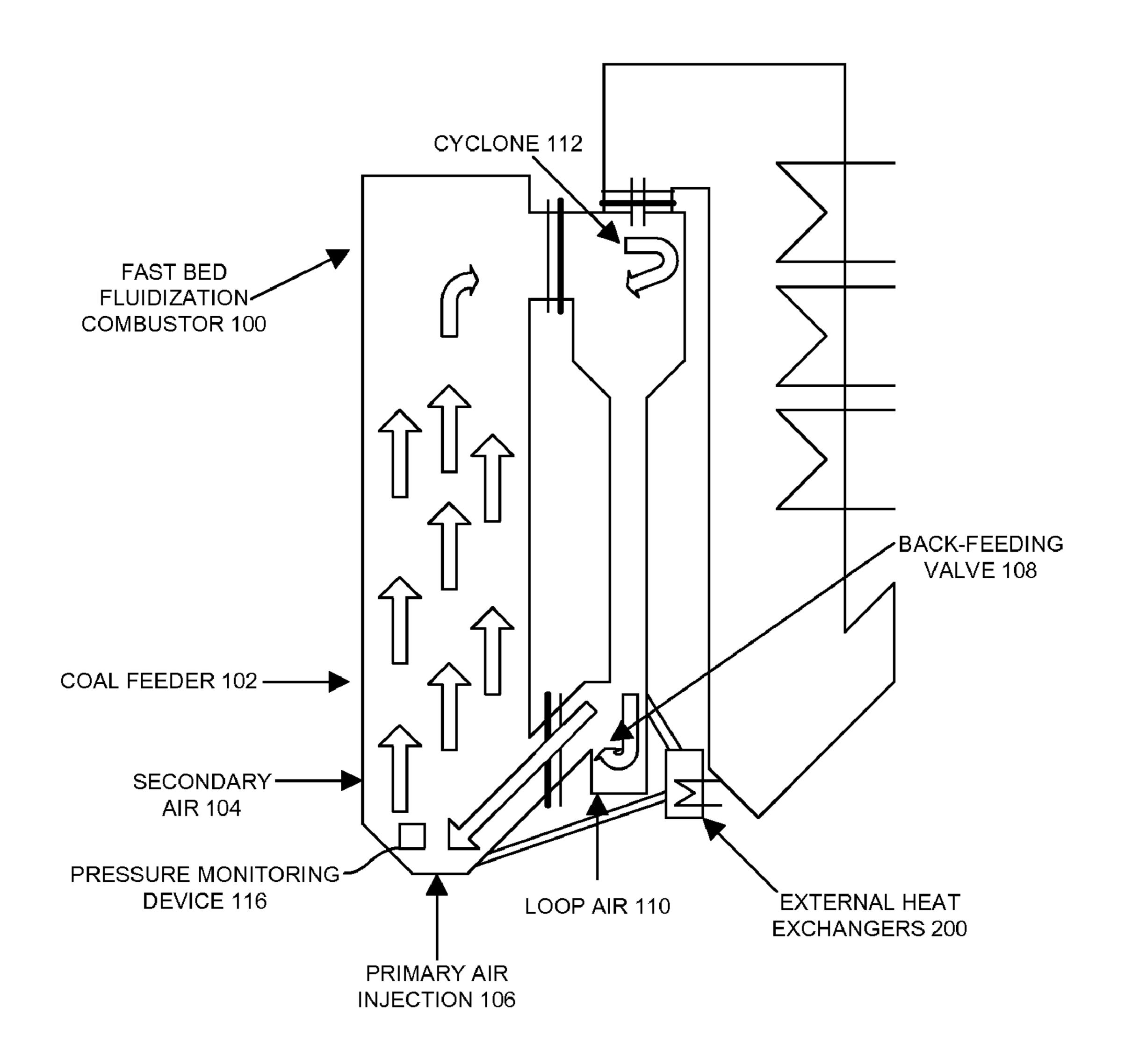
**CFB BOILER WITH HEAT EXCHANGE 250**
