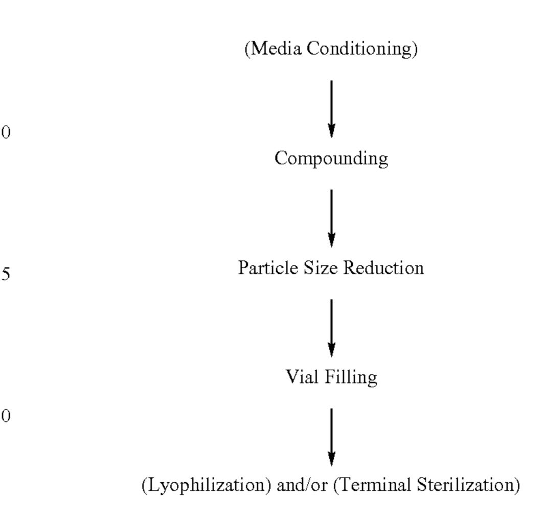
As indicated by the optional steps in parentheses, some of the processing is dependent upon the method of particle size reduction and/or method of sterilization. For example, media conditioning is not required for a milling method that does not use media. If terminal sterilization is not feasible due to chemical and/or physical instability, aseptic processing can be used.
