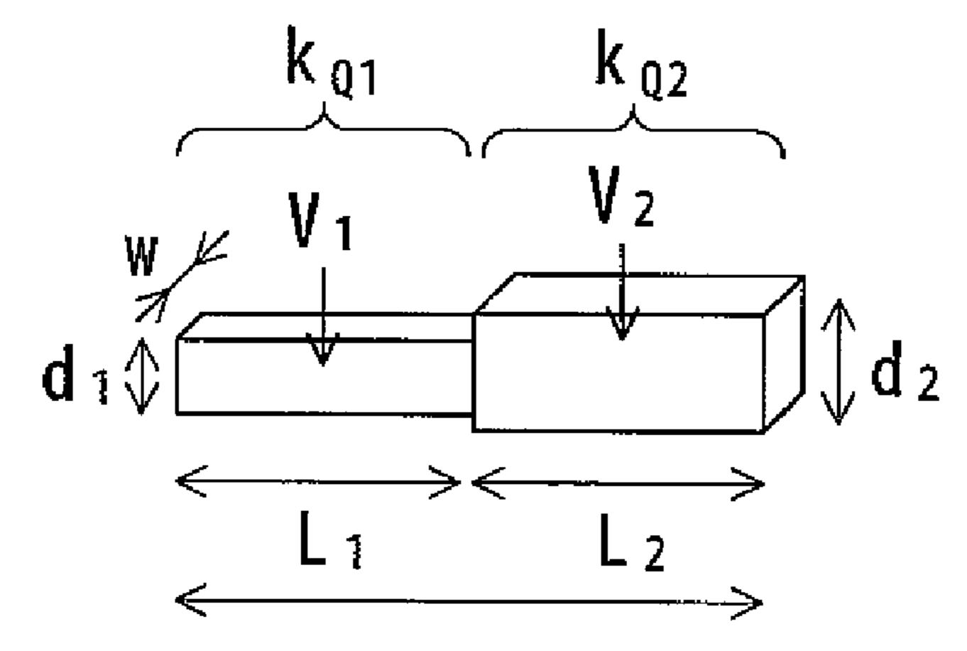
PRESSURE DROP P AND VOLUME V ARE CONSTANT  $(V = V_1 + V_2)$
