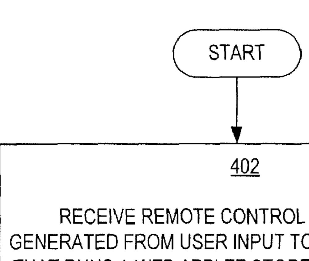
RECEIVE REMOTE CONTROL COMMANDS GENERATED FROM USER INPUT TO A SMART PHONE THAT RUNS A WEB APPLET STORED ON COMPUTER READABLE MEDIA COMMUNICATIVELY COUPLED TO THE SMART PHONE
