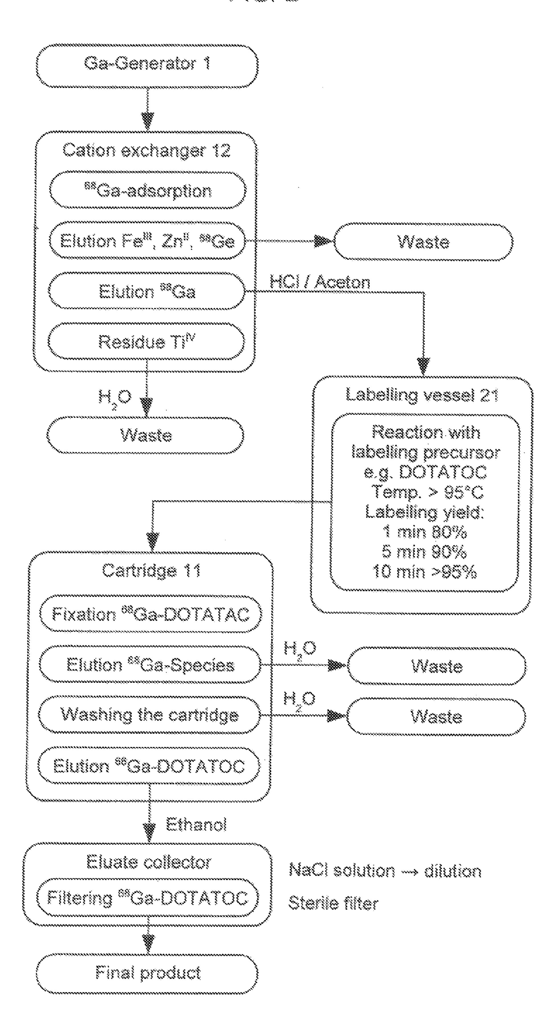
METHOD AND DEVICE FOR ISOLATING A CHEMICALLY AND RADIOCHEMICALLY CLEANED <sup>68</sup>GA-RADIONUCLIDE AND FOR MARKING A MARKING PRECURSOR WITH THE <sup>68</sup>GA-RADIONUCLIDE
