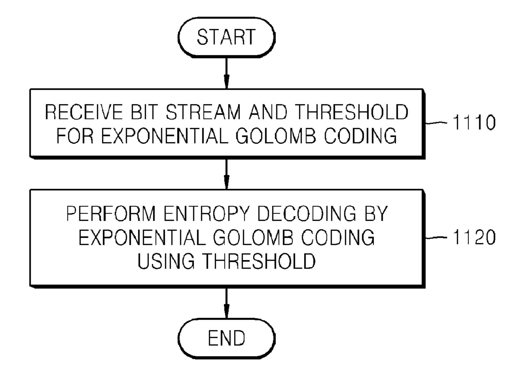
METHOD AND APPARATUS FOR ENCODING IMAGE BY EXPONENTIAL GOLOMB BINARIZATION USING OPTIMAL THRESHOLD, AND METHOD AND APPARATUS FOR DECODING IMAGE BY **EXPONENTIAL GOLOMB BINARIZATION** USING OPTIMAL THRESHOLD
