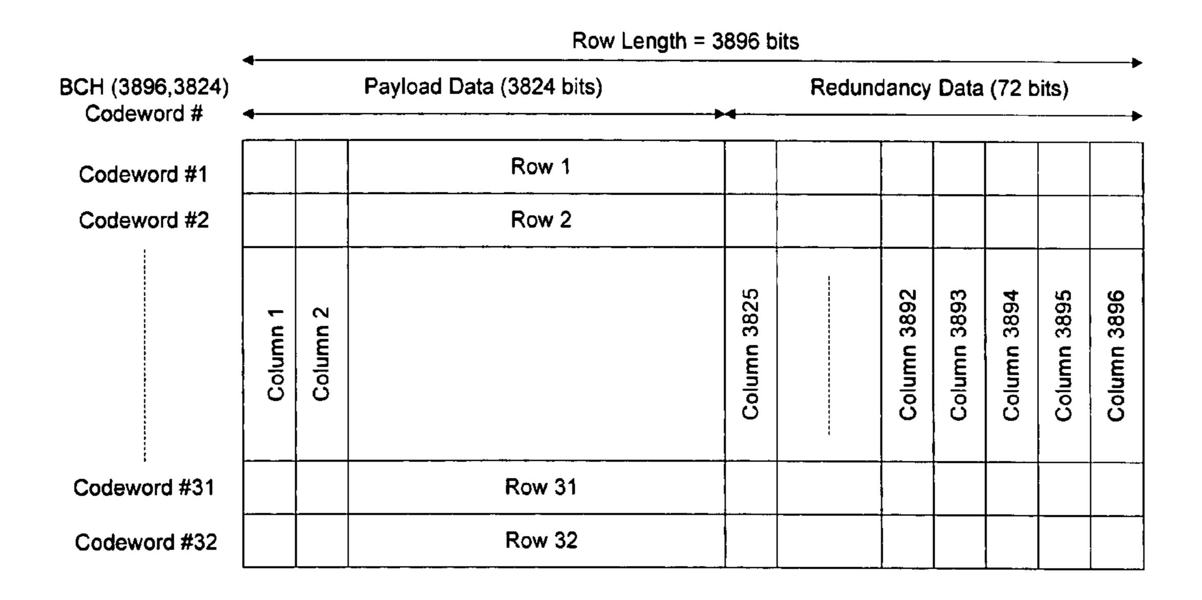
Figure 2: Intermediate Frame Format
