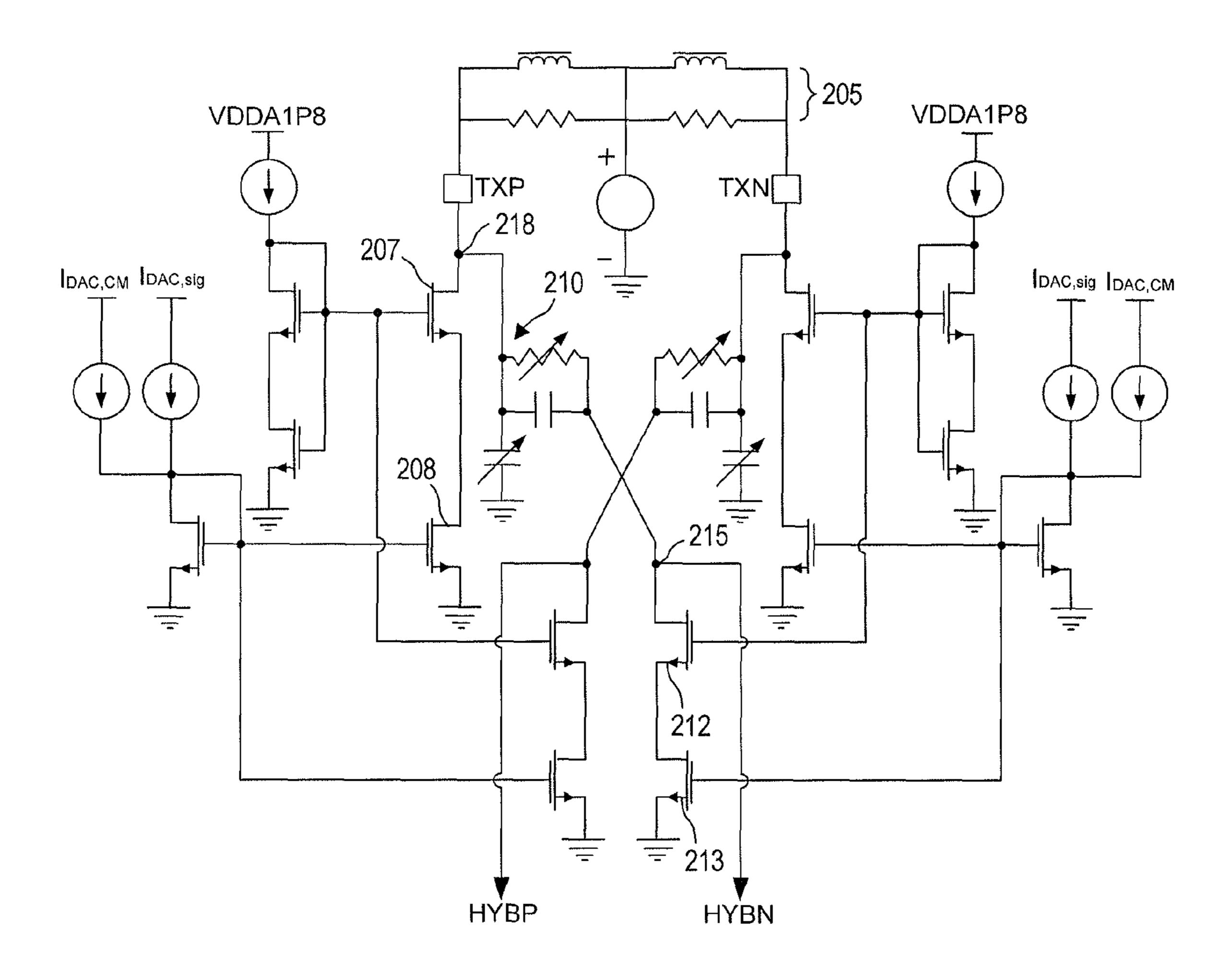
Figure 2. Schematic Representation of the Preferred Embodiment
